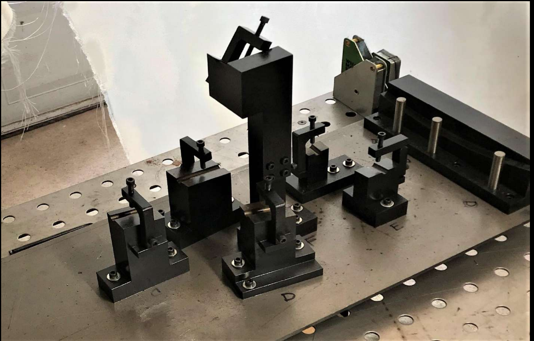
Completed Leg Fixture Clamps: Like the fixture positioning blocks, I had all of the leg fixture clamps coated in black oxide to prevent rust as well.
