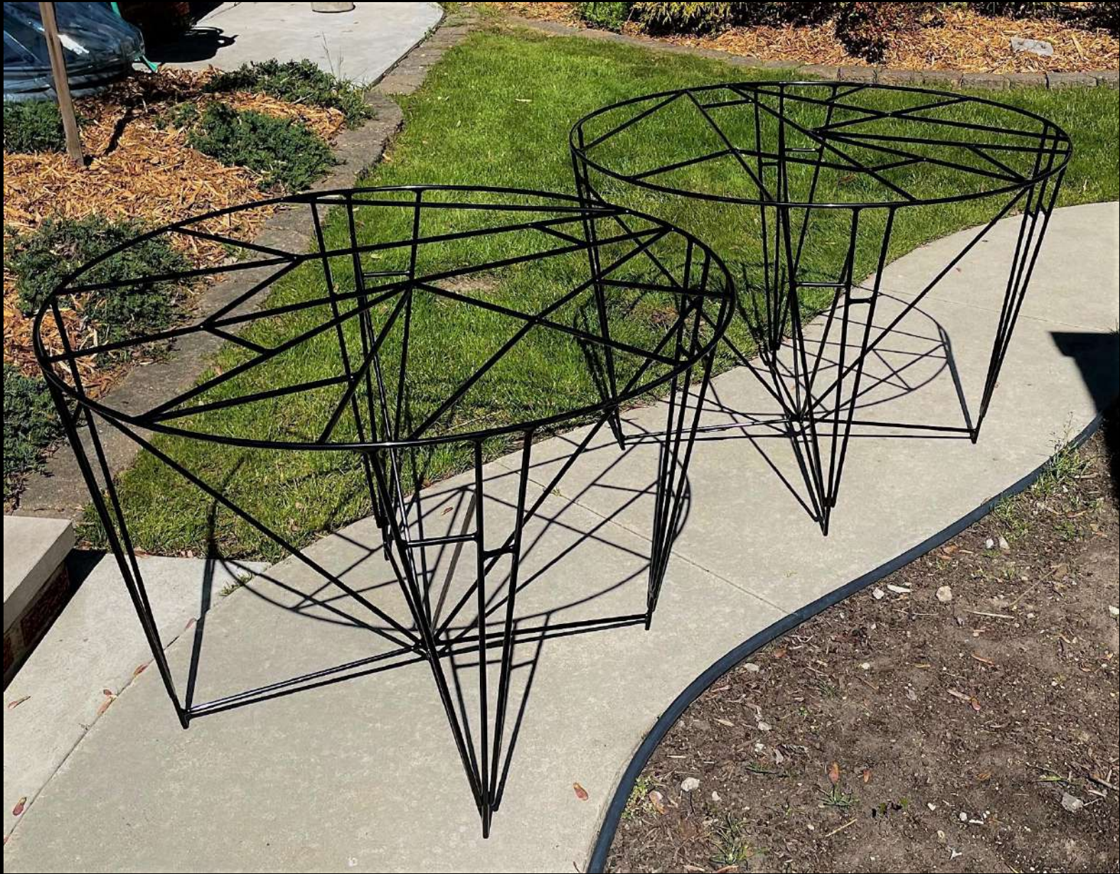
Powder Coated Tables ISC-00001 & ISC-00002: Powder coating is complete. My tables have been powder coated in the gloss black color that was selected.
