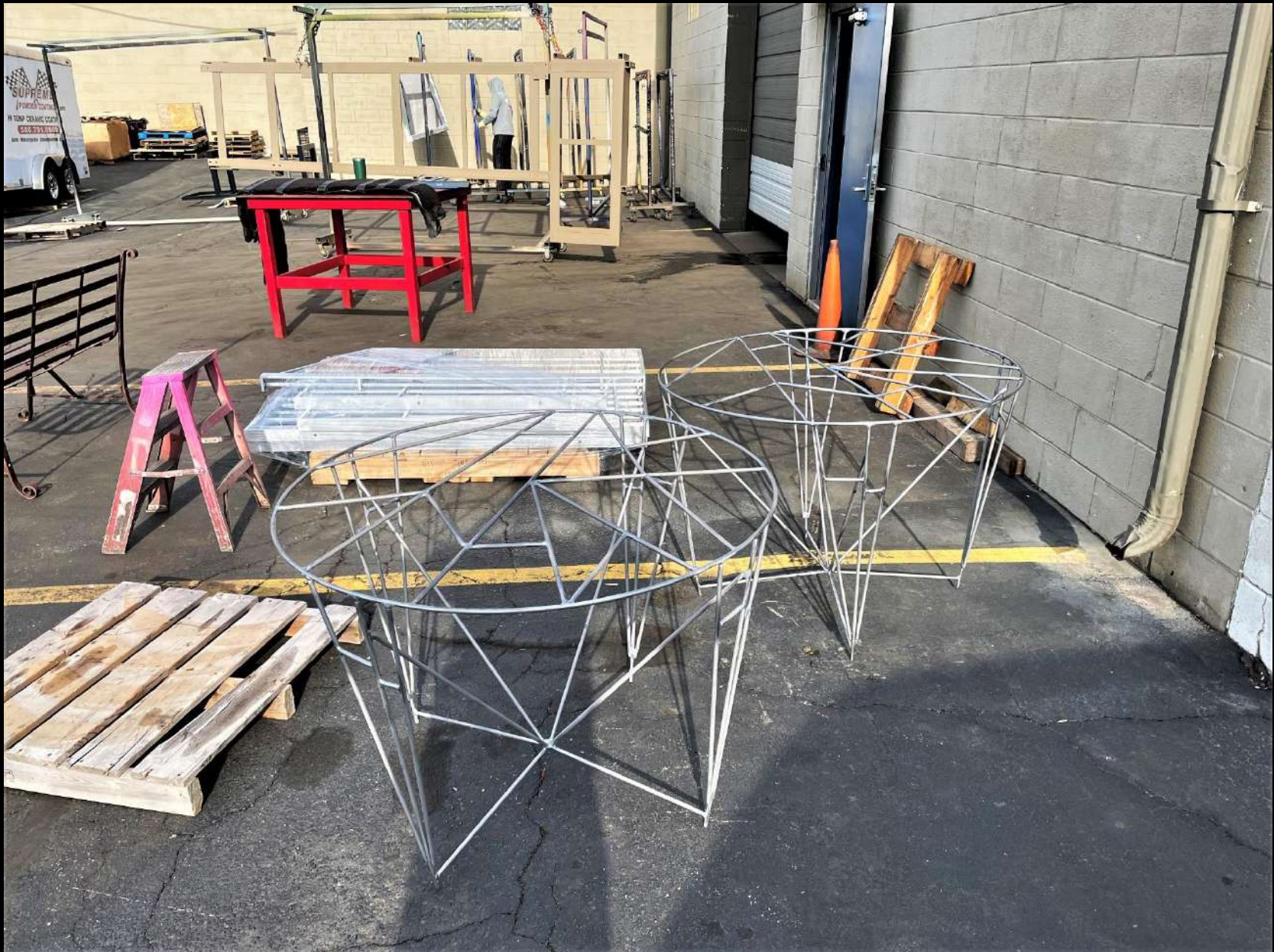
Powder Coating Tables ISC-00001 & ISC-00002: Time to powder coat. I have delivered my two tables to the powder coating vendor to get coated and baked in the oven.
