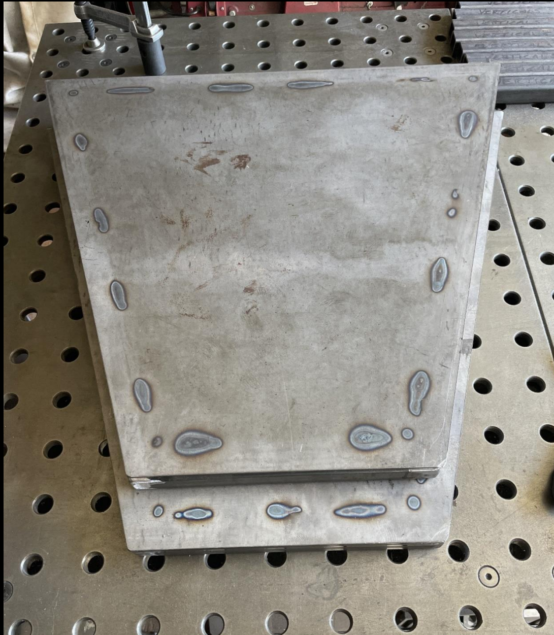
Both table tops and top table frames have been welded together.
