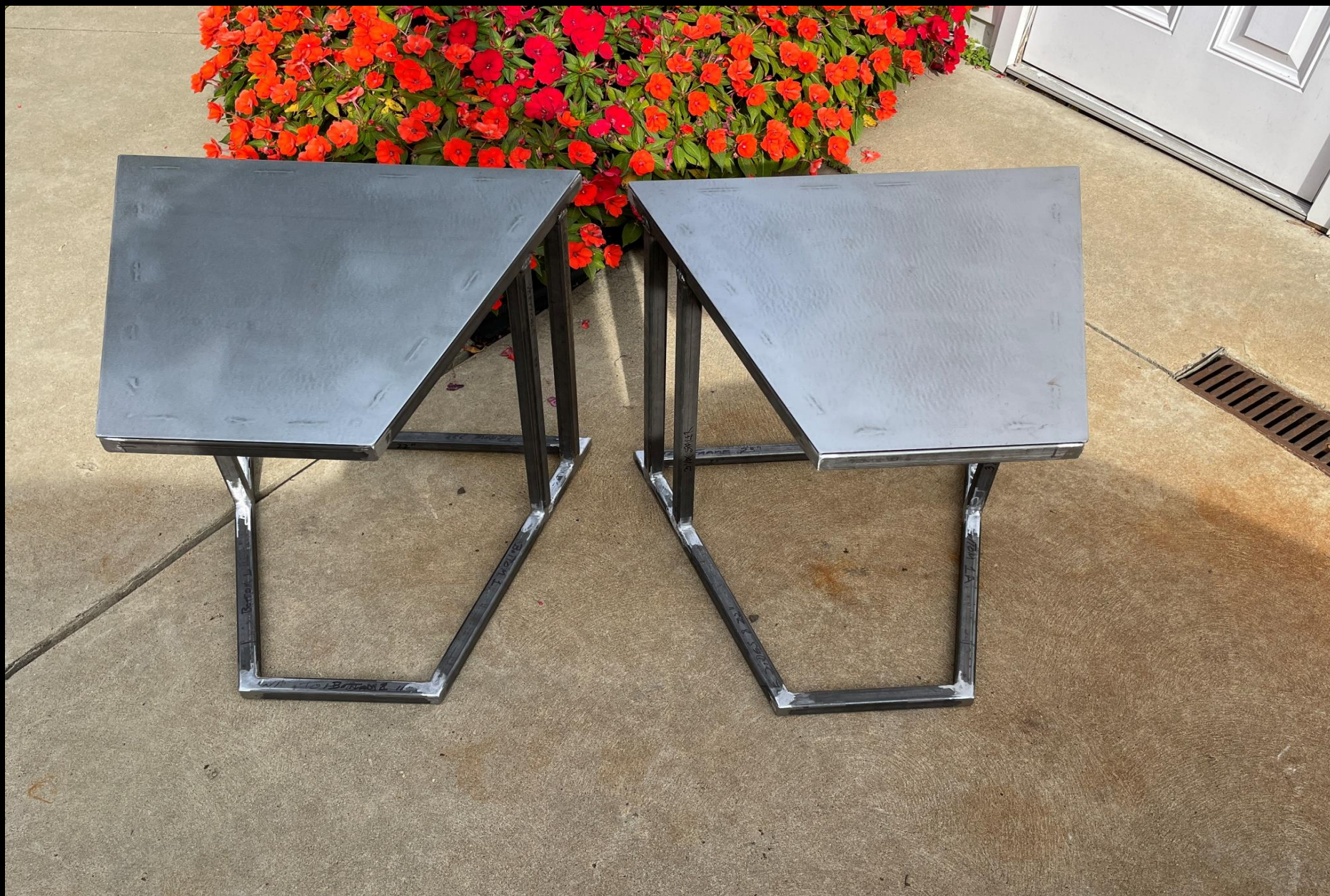
The Trapezoid Coffee Tables are now finished and ready to go to powder coating.
