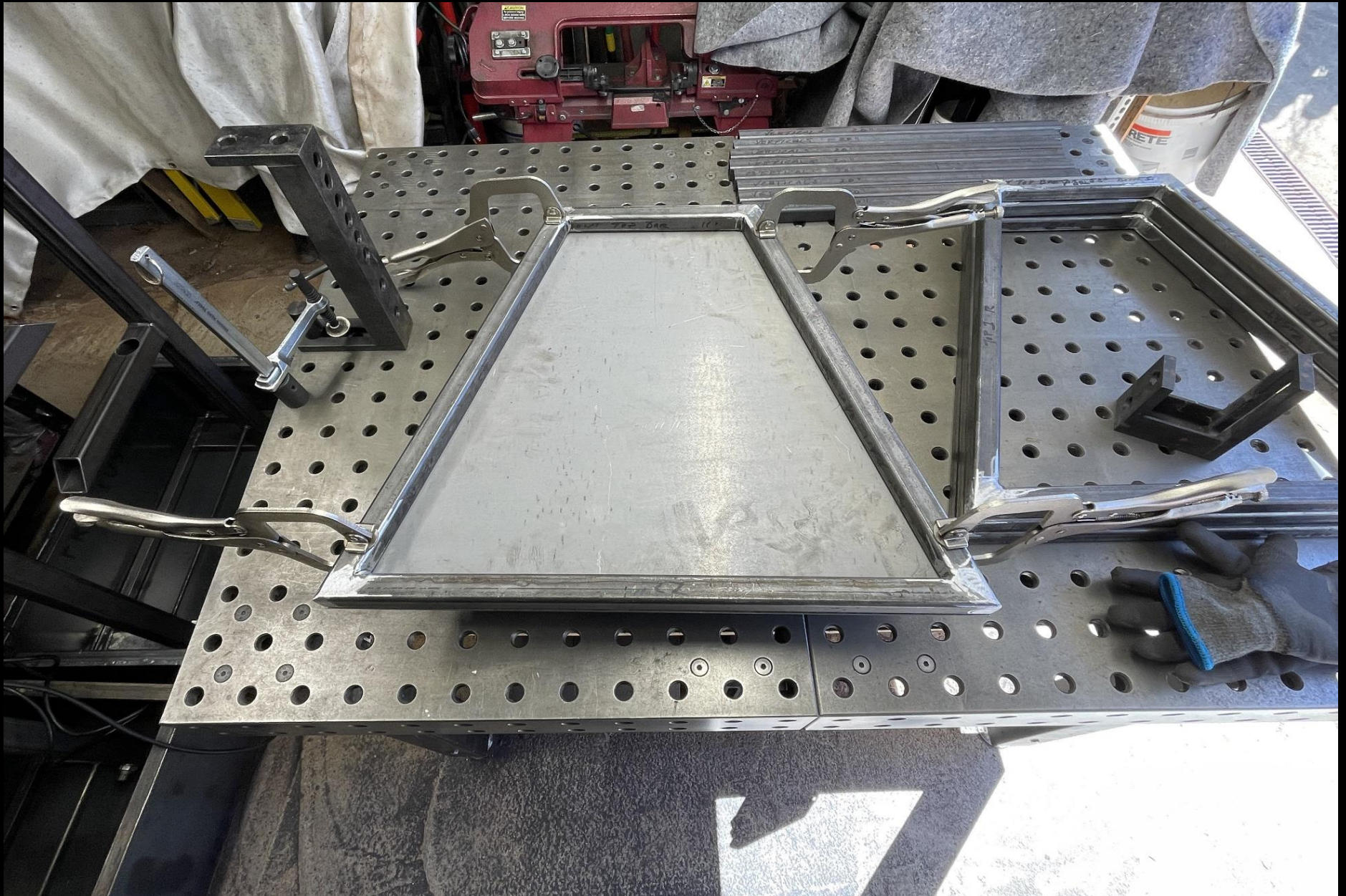
The finish ground top frame is mated to the table top and clamped in place for welding.
