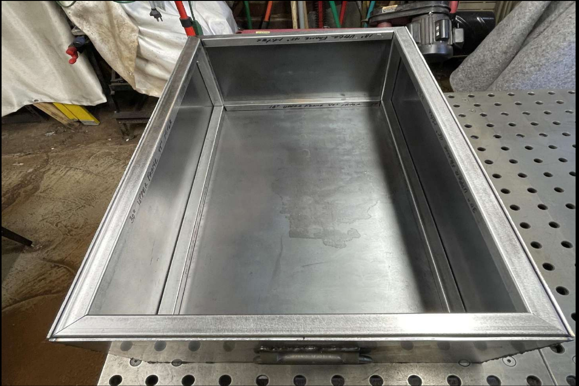
Here is the tank box frame fitted inside the steel tank. The frame fits in nicely with a few minor adjustments.
