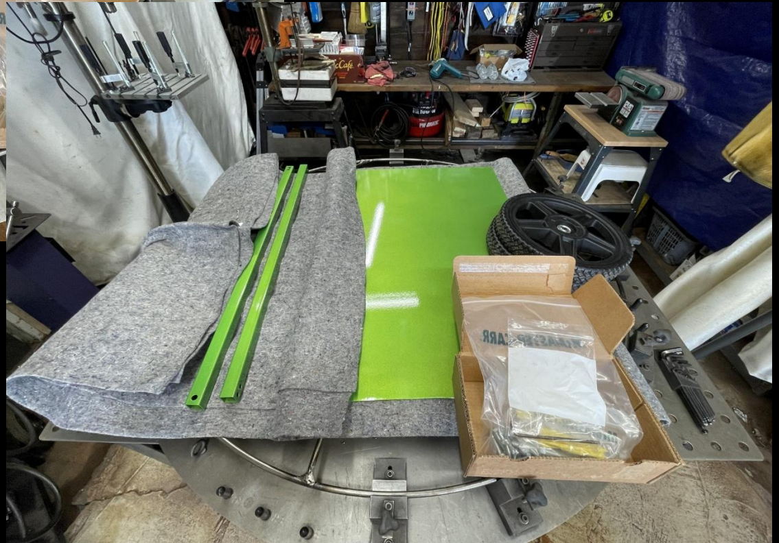
The Patio Bar Cart handle, shelves and cross rails after powder coating.
