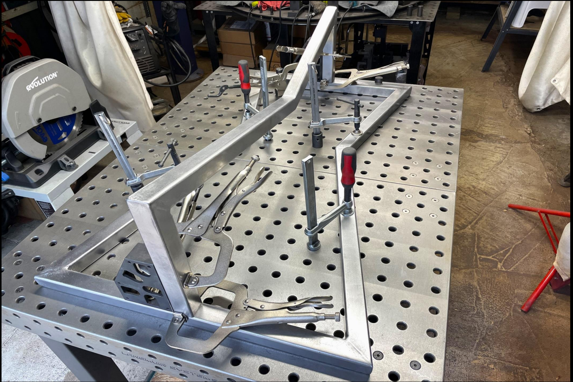
This is the setup that I used to attach the first split to each of my tables, making sure the split is on center, top to top and base to base.
