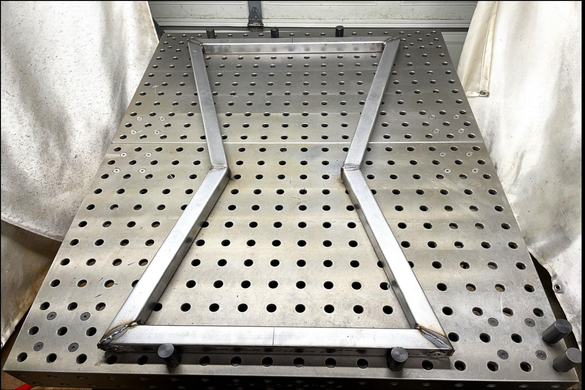
Base for Table 1, 'A' side welds on miter joints complete.
