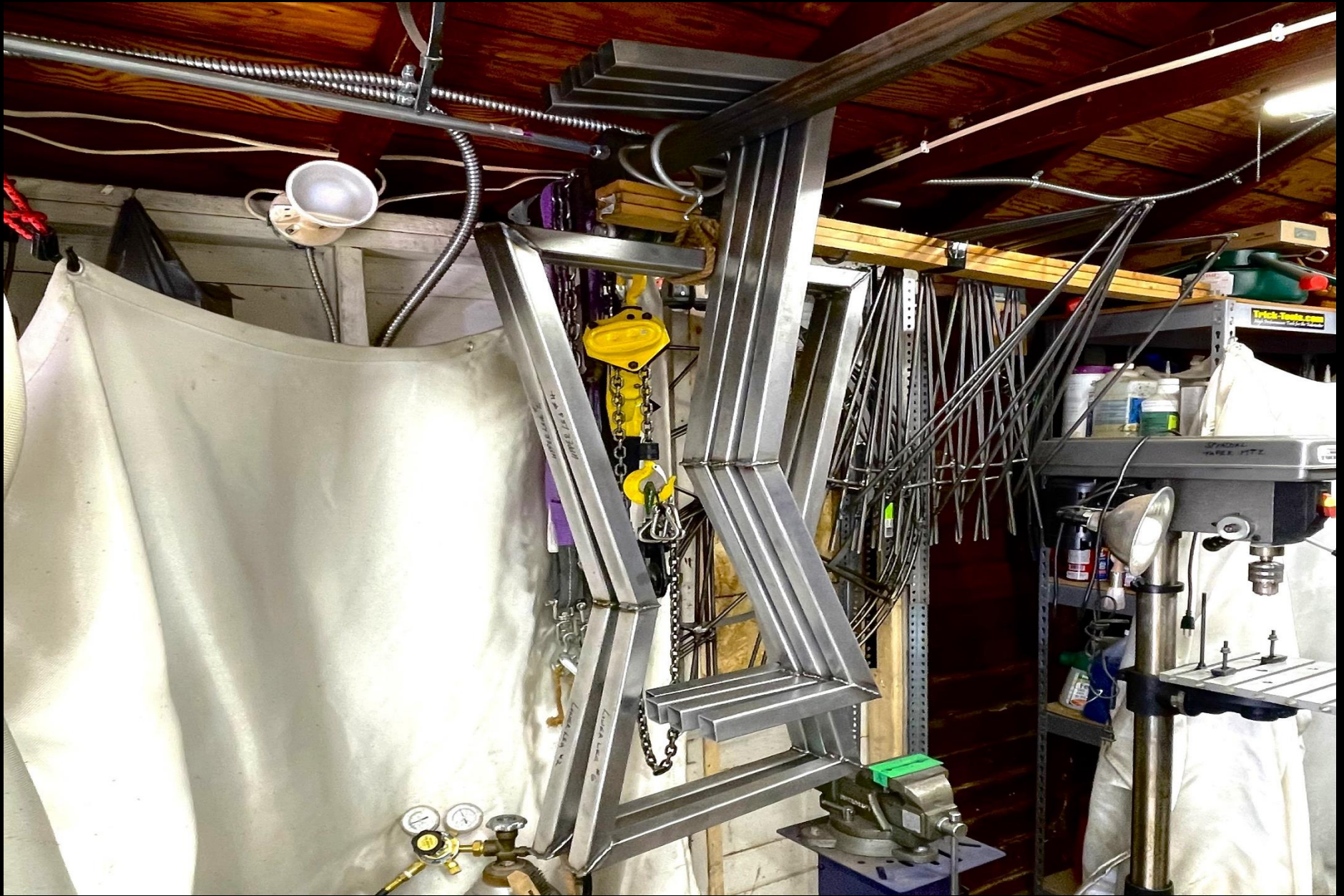
The two component bases and four splits are welded.
