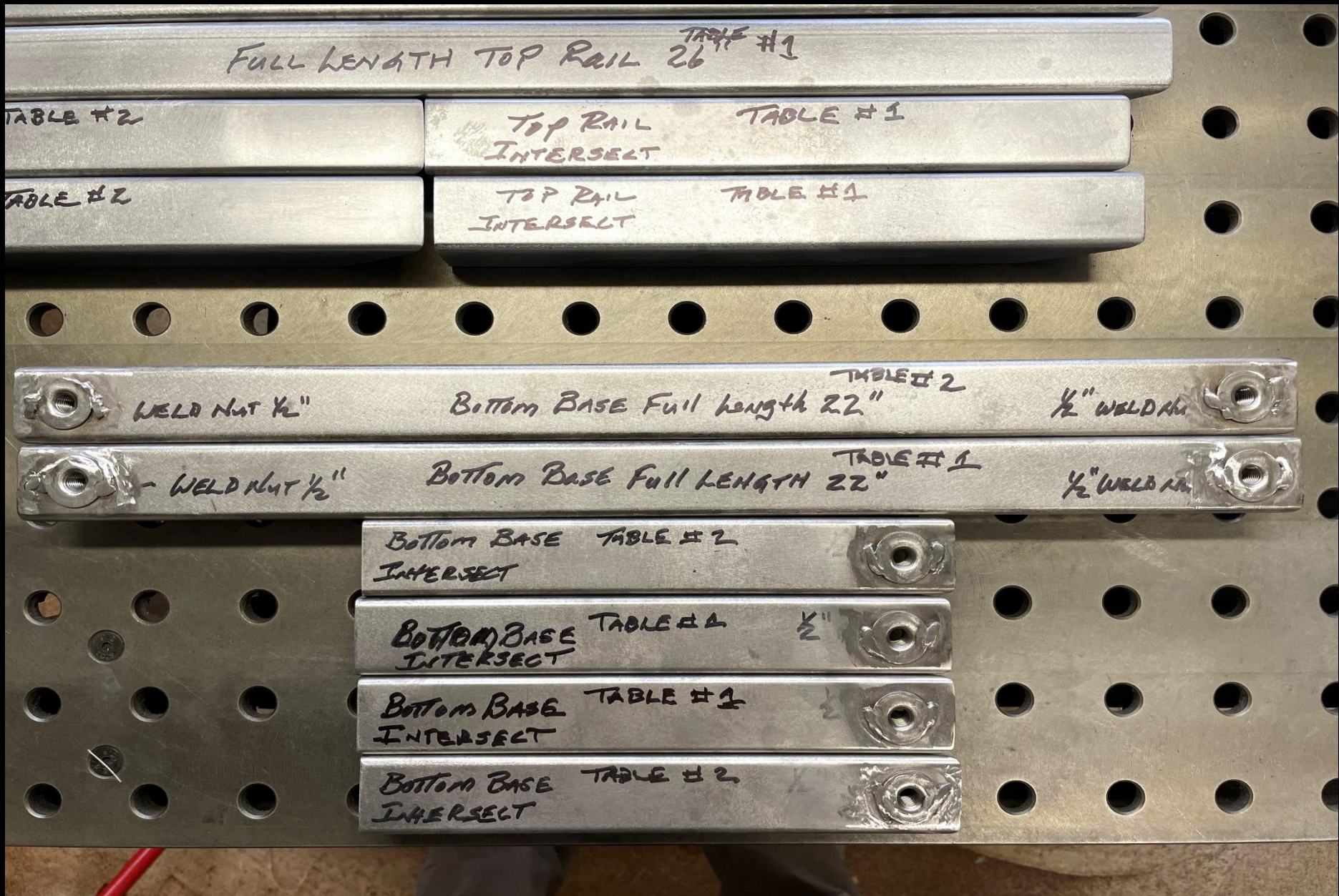
The bottom two base rails and the half split components all have the weld nuts in place.
