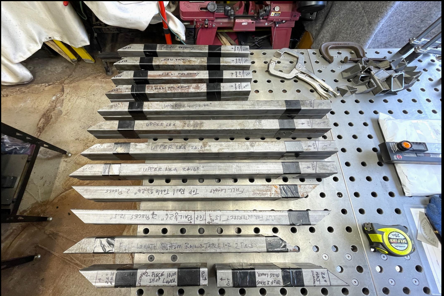
All of the 35.5 degree miter cuts are completed to make the two tables.
