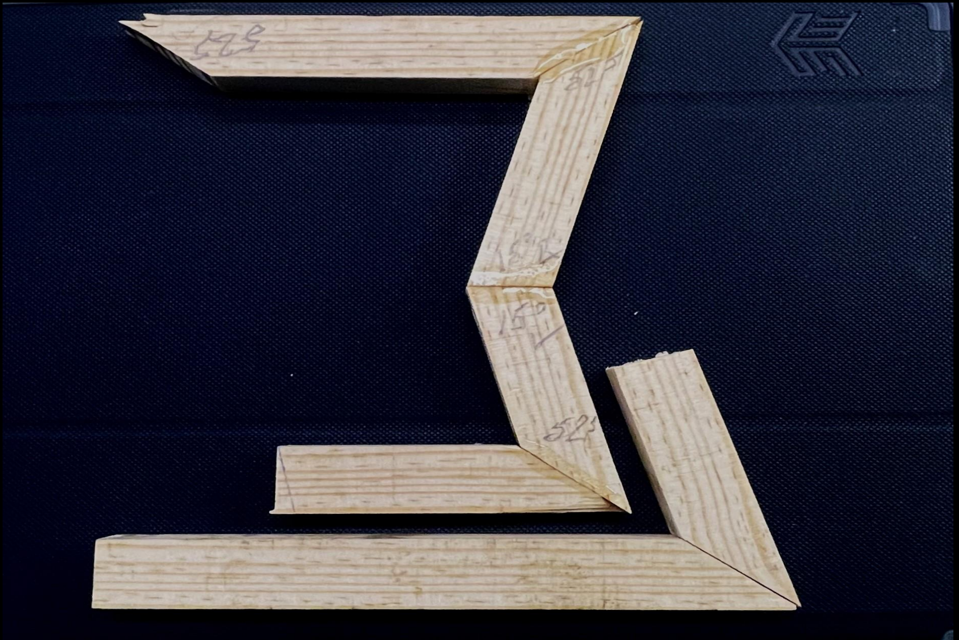
Prototype Mockup of Monaco Table Base Miter Cuts: Miter saw setup requires 35.5 degree mating angles on the top and bottom and 15 degree mating angles in the center.
