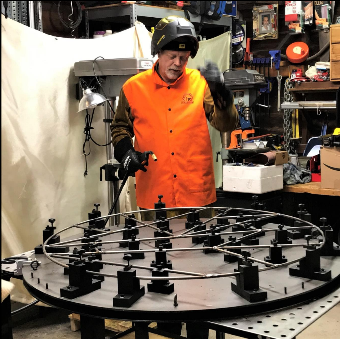
Welding The "A" & "B" Side Table Top Interior Design: After I custom fit each rod segment into its designated position for the interior design, it's time to weld the table top "A" side.
