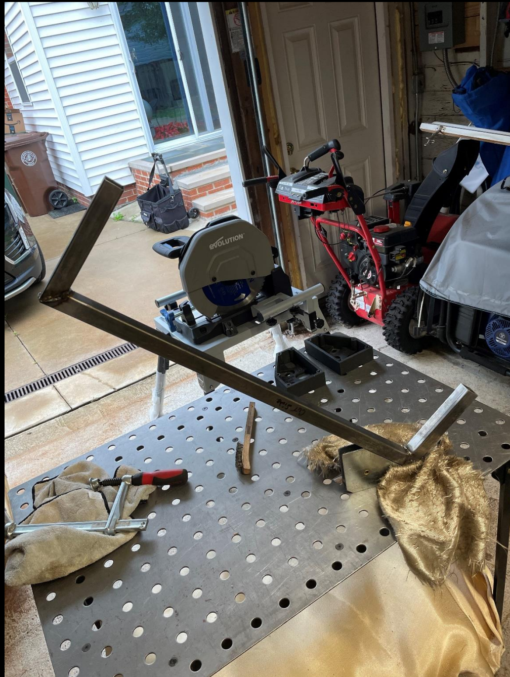
Spa Book Shelf- Fabrication Sequence: 6 Welding the inside angle on shelf.
