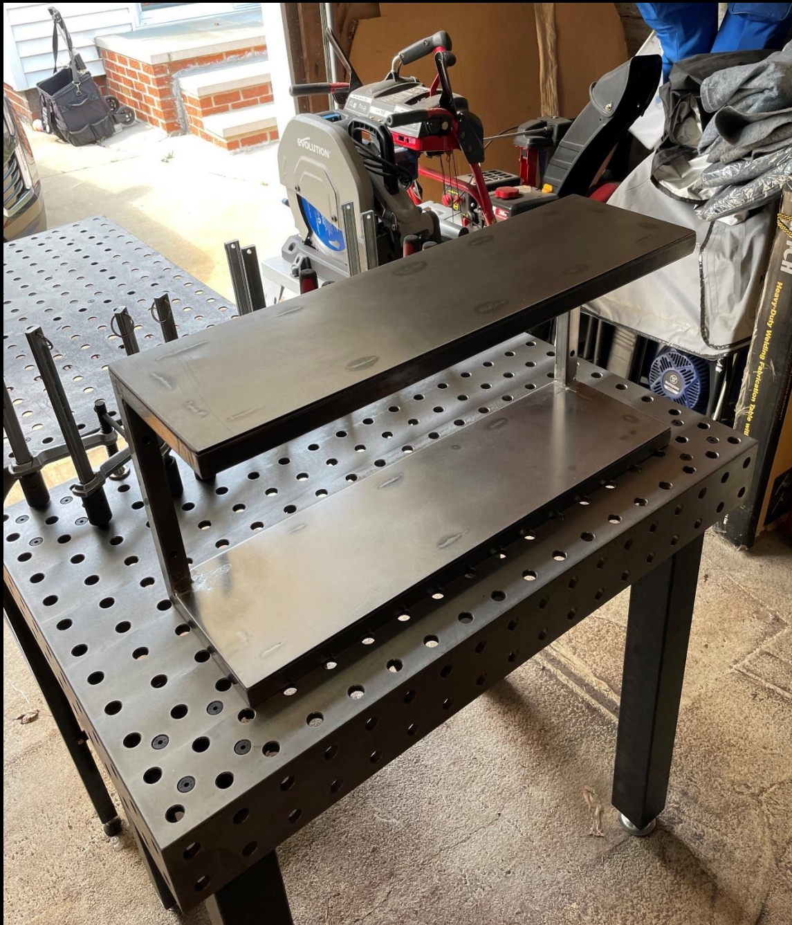
Spa Book Shelf- Fabrication Sequence: 30 Finish grind and sand top & bottom plates.
