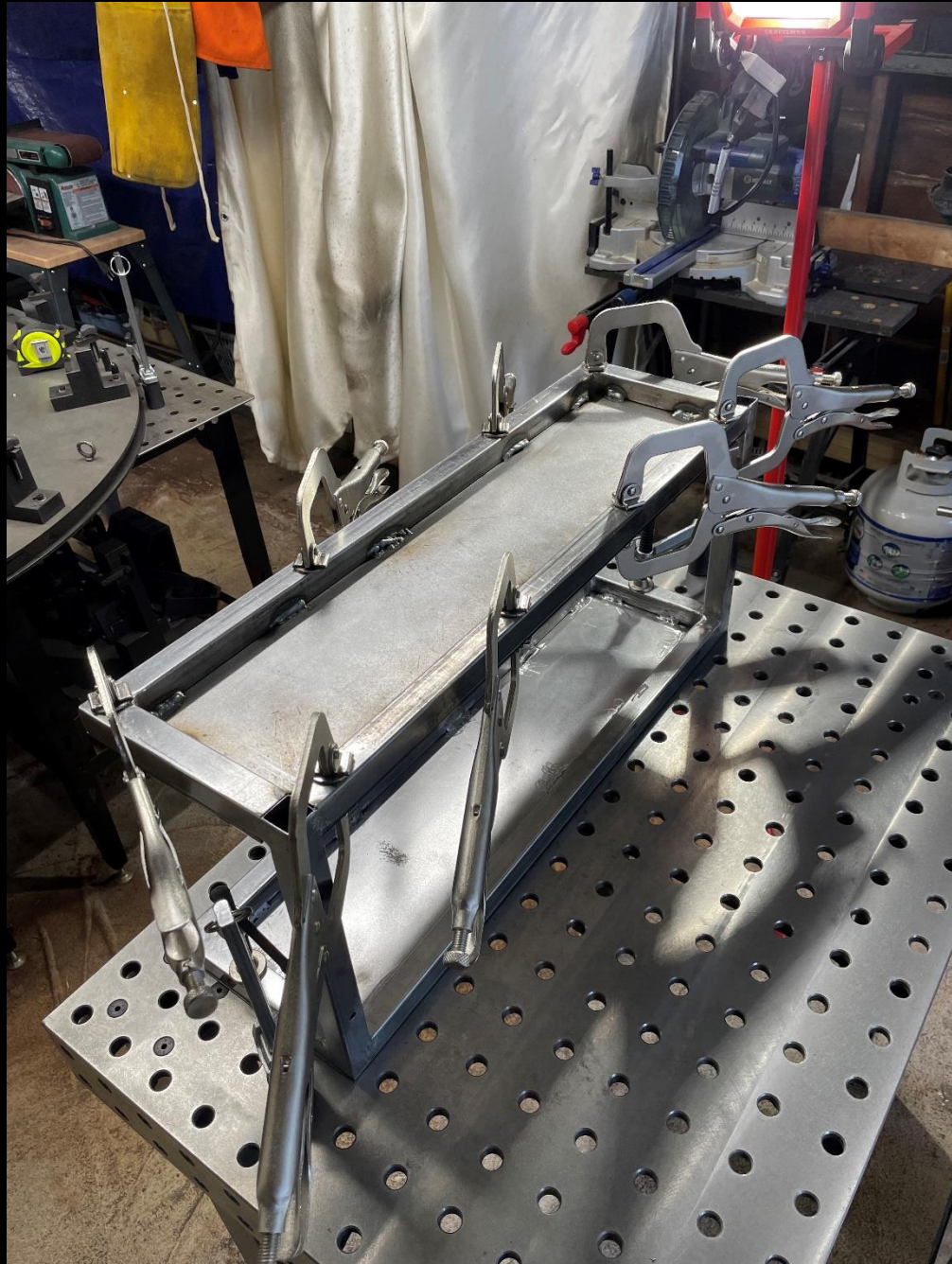
Spa Book Shelf- Fabrication Sequence: 27 Bottom plate is positioned, clamped & welded.
