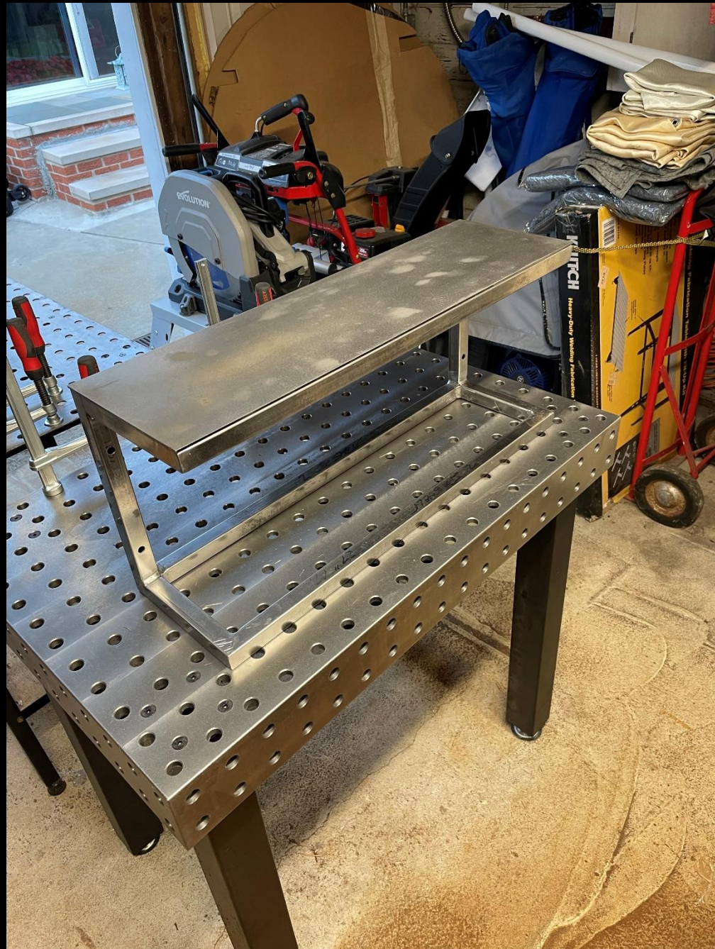
Spa Book Shelf- Fabrication Sequence: 22 Evaluating fit & positioning of top plate.
