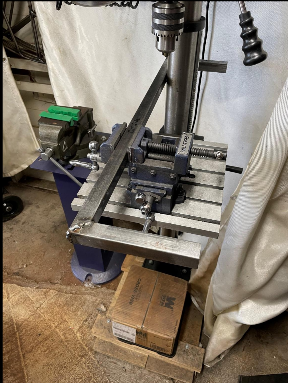
Spa Book Shelf- Fabrication Sequence: 10 Clean up welds on shelf frame.
