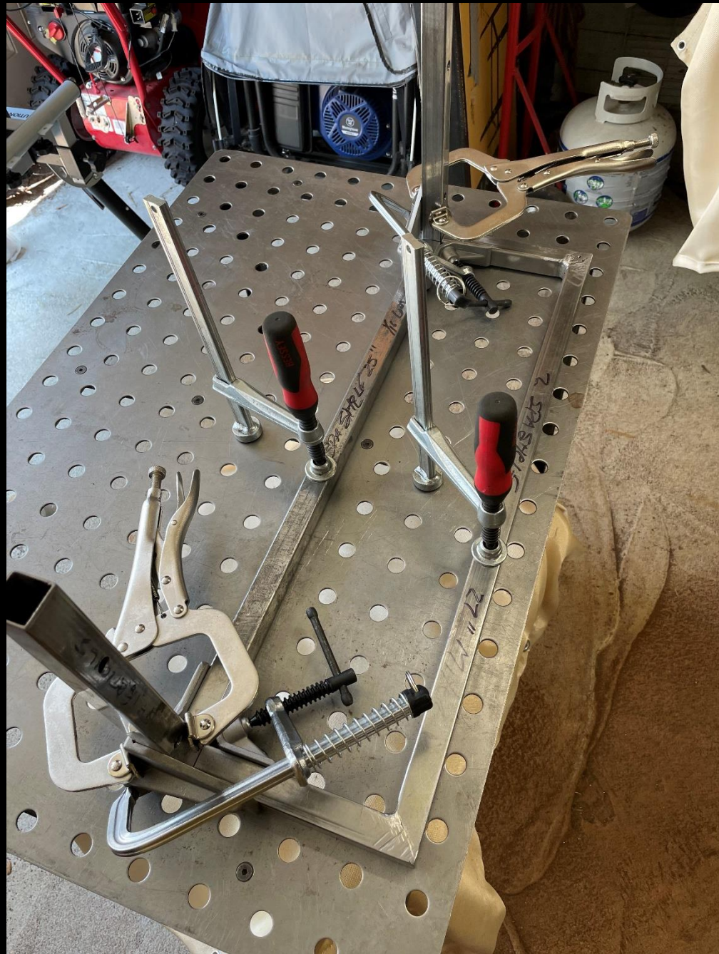
Spa Book Shelf- Fabrication Sequence: 13 Tack weld vertical legs & back rail.
