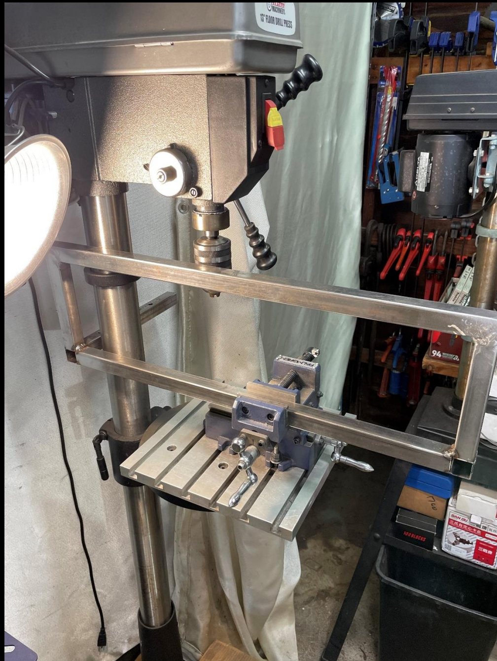
Spa Book Shelf- Fabrication Sequence: 15 Clean up welds on lower shelf frame.
