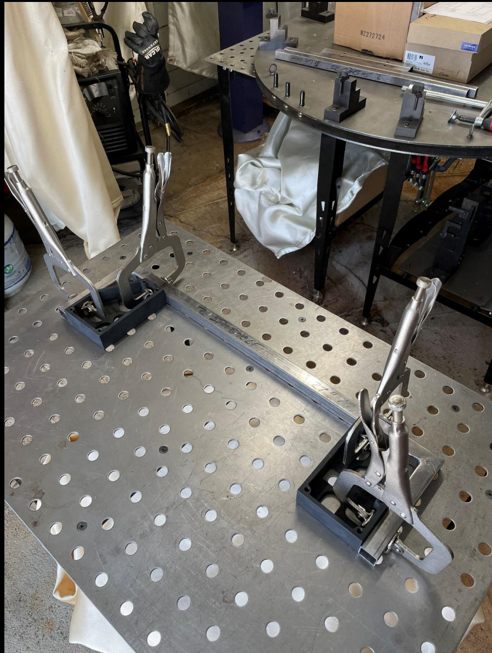
Spa Book Shelf- Fabrication Sequence: 3 Welding miter cuts for shelf brackets.
