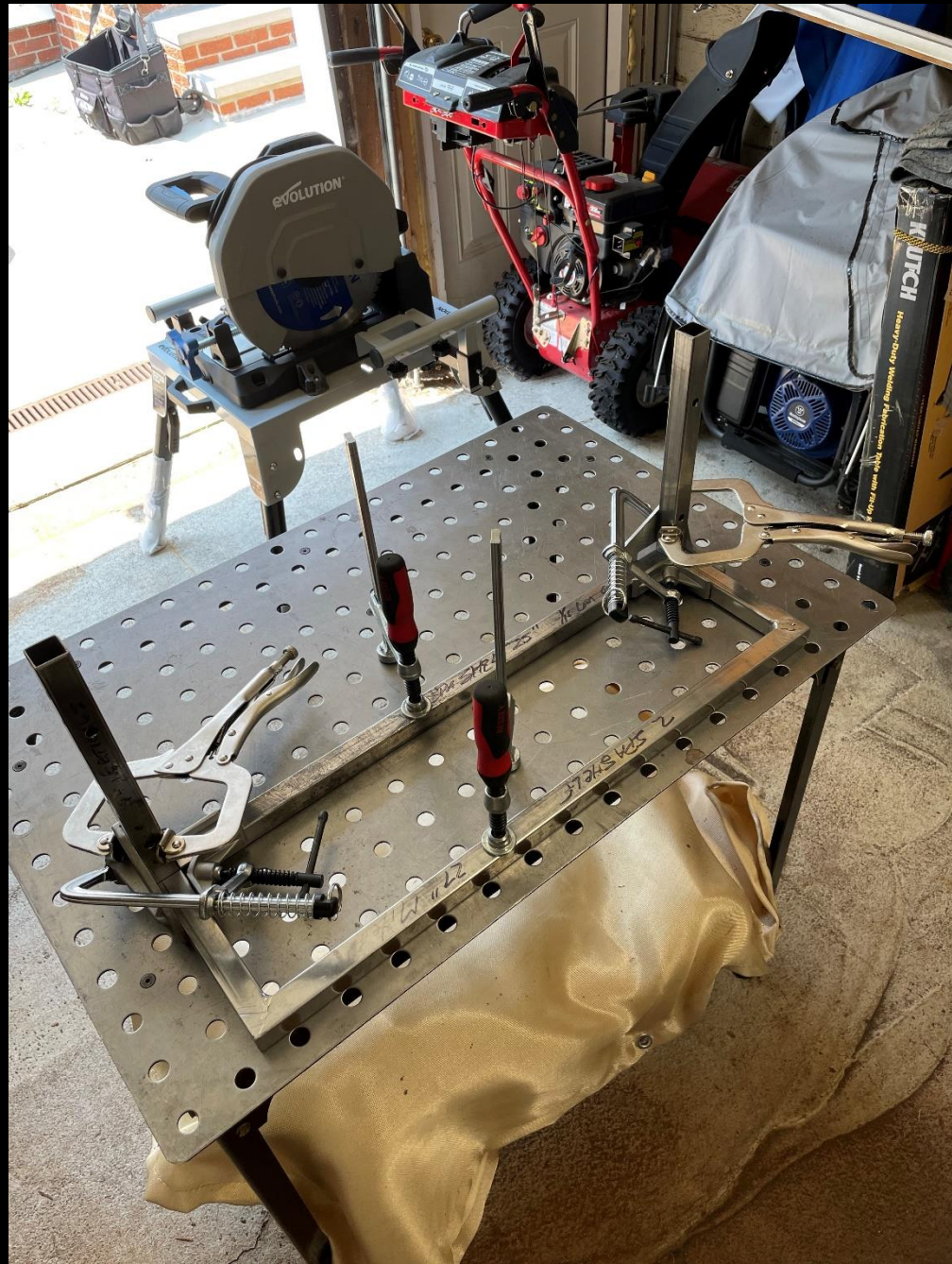
Spa Book Shelf- Fabrication Sequence: 11 Weld vertical legs & shelf back-lower.
