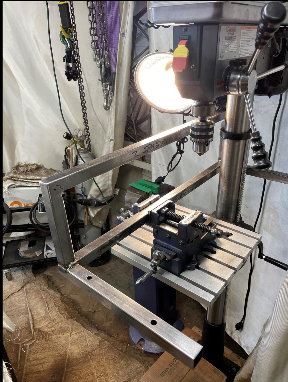
Spa Book Shelf- Fabrication Sequence: 16 Clean up welds on shelf frame.
