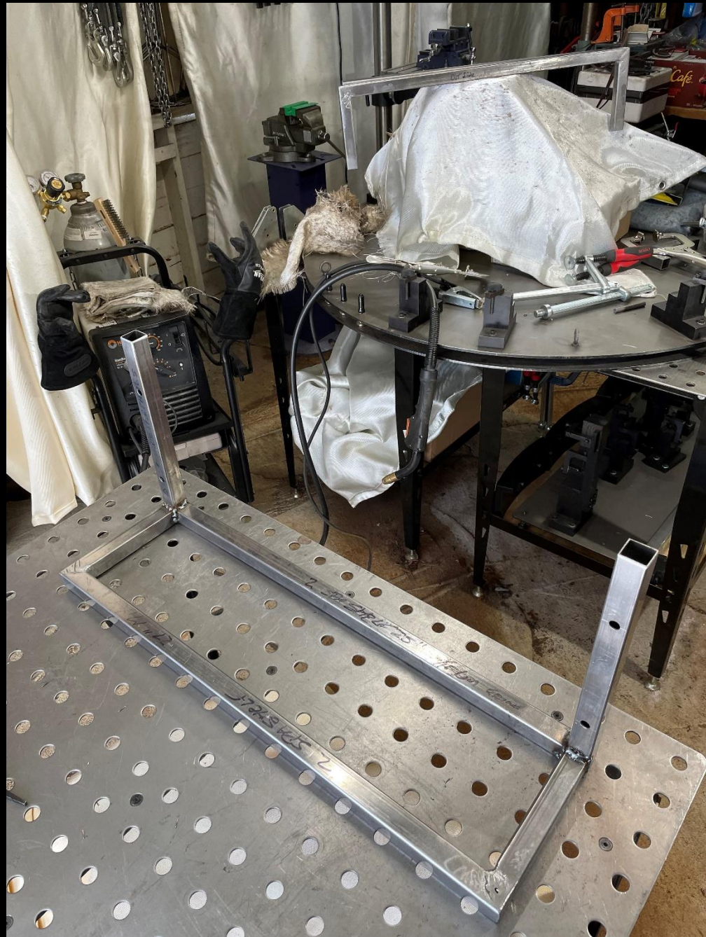
Spa Book Shelf- Fabrication Sequence: 14 Finished welds on lower shelf frame.
