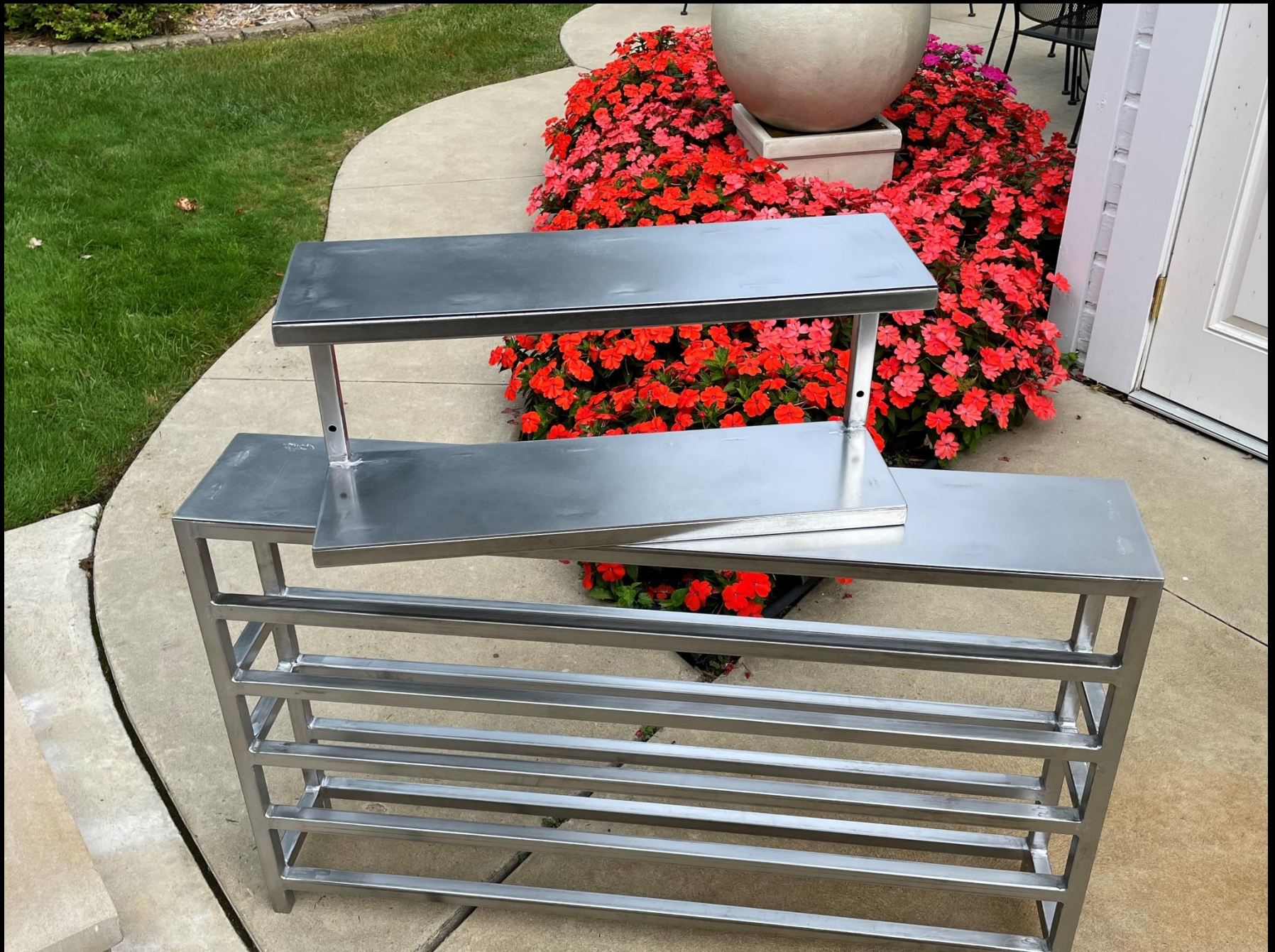
Spa Book Shelf- Fabrication Sequence: 31 The spa shelf ready for powder coating.
