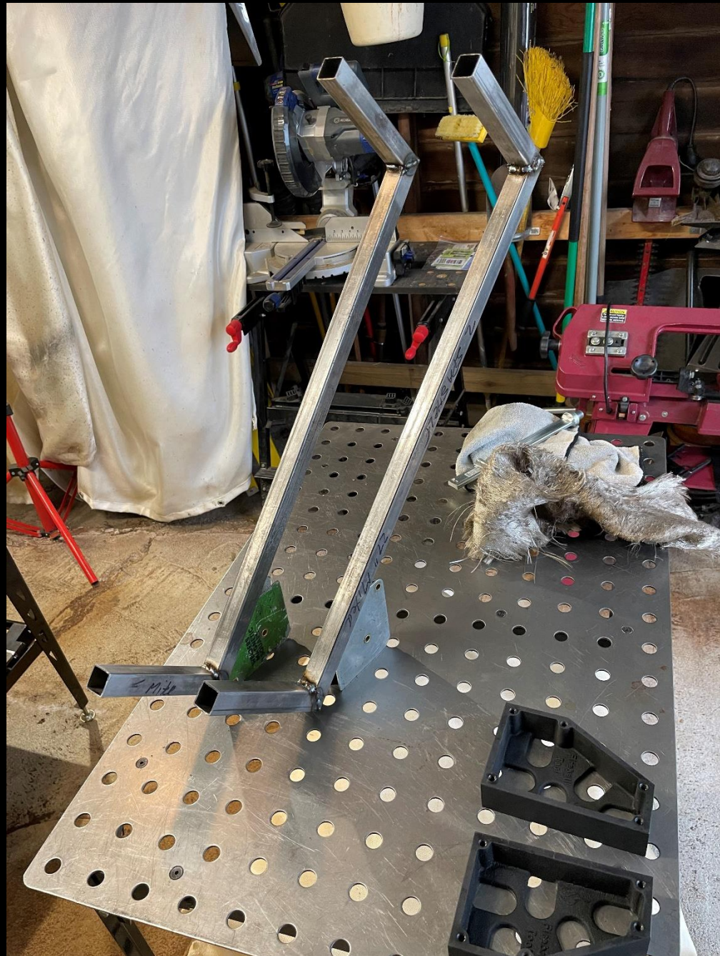
Spa Book Shelf- Fabrication Sequence: 8 Welding complete on inside angles.
