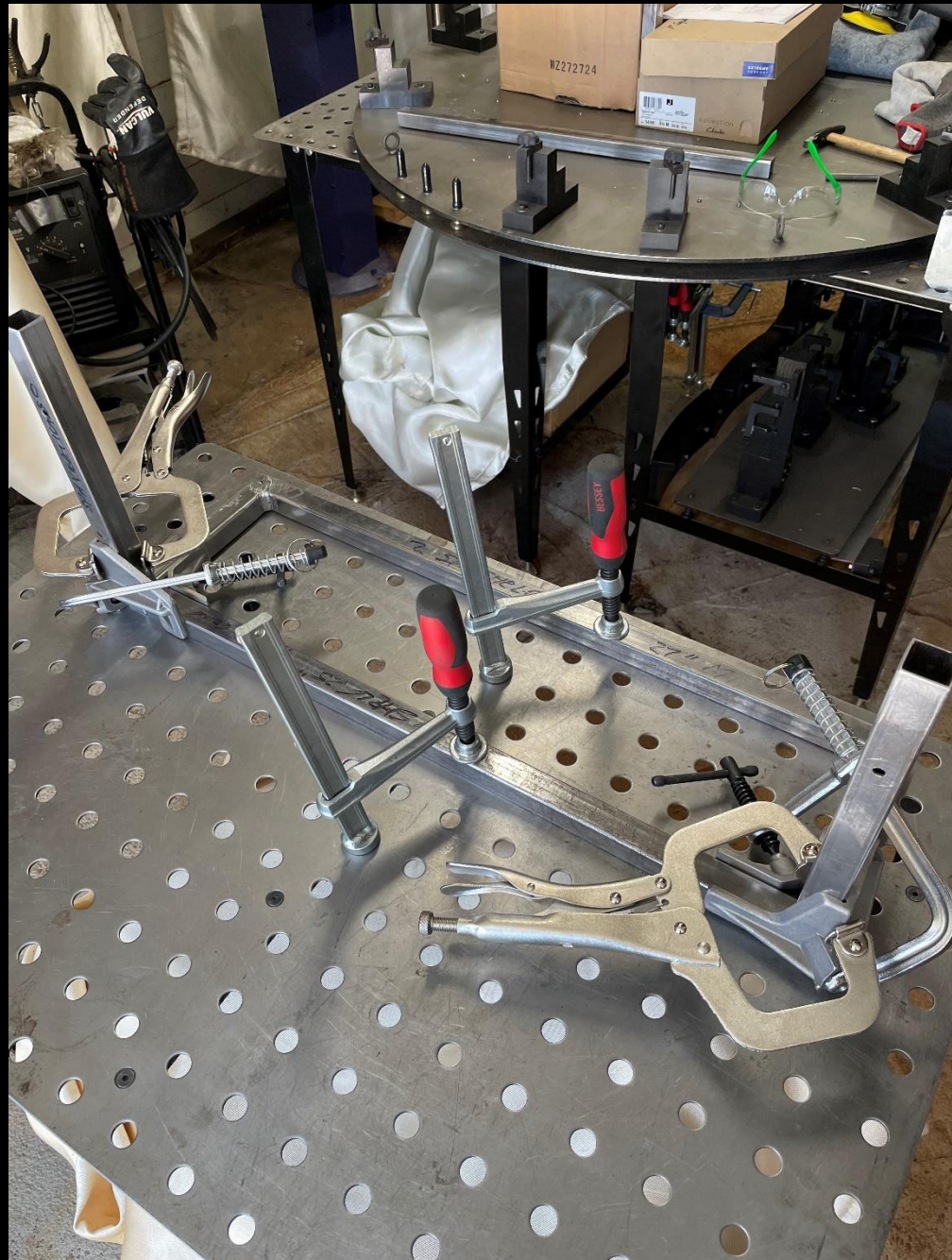
Spa Book Shelf- Fabrication Sequence: 12 Using 3 axis clamps to position verticals.
