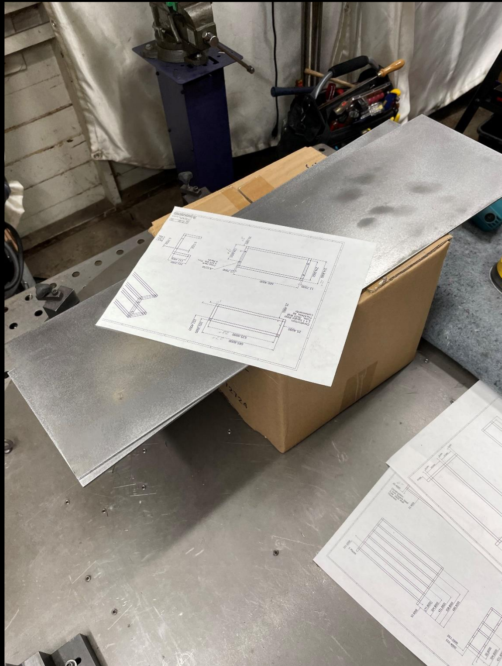
Spa Book Shelf- Fabrication Sequence: 21 Laser cut top & bottom plates.
