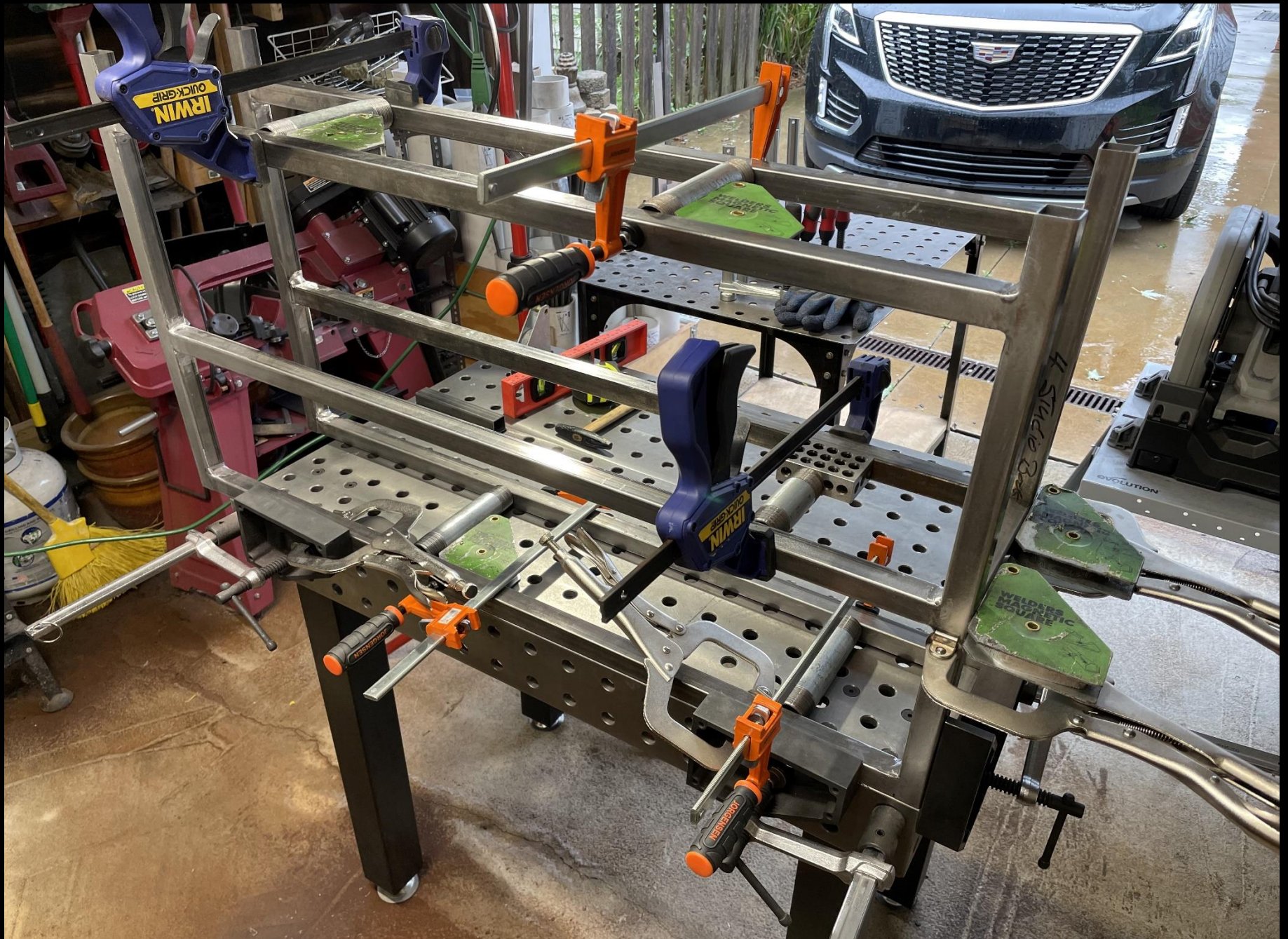
Fabrication Sequence: 10 A number of clamps & spacers are required to align the panels.
