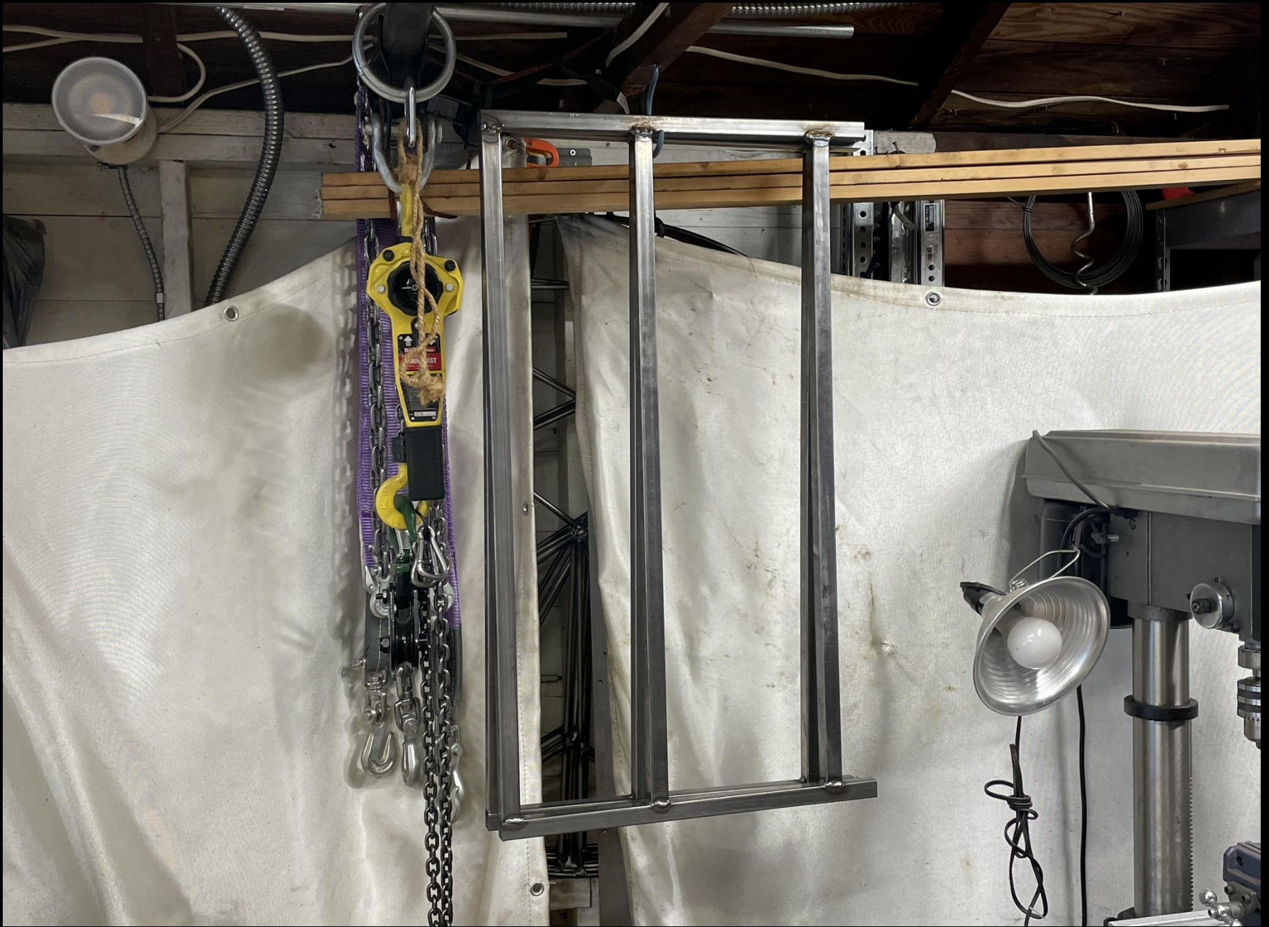
Fabrication Sequence: 8 After welding the panels, the welds need to be ground & finished.
