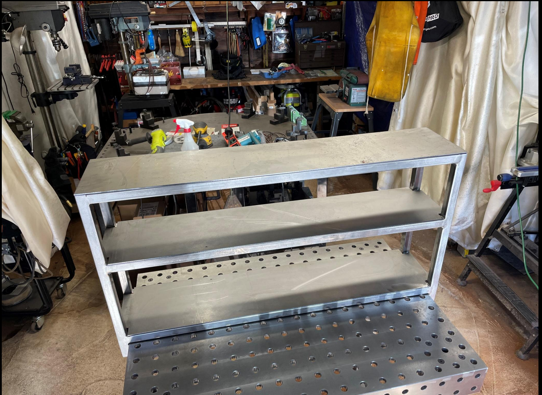
Fabrication Sequence: 20 Plate welds are ground and the steel plates sanded.
