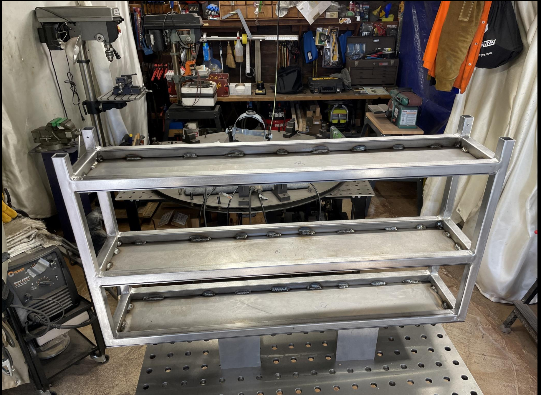
Fabrication Sequence: 18 Top, mid & bottom plates are clamped and welded to the frame.
