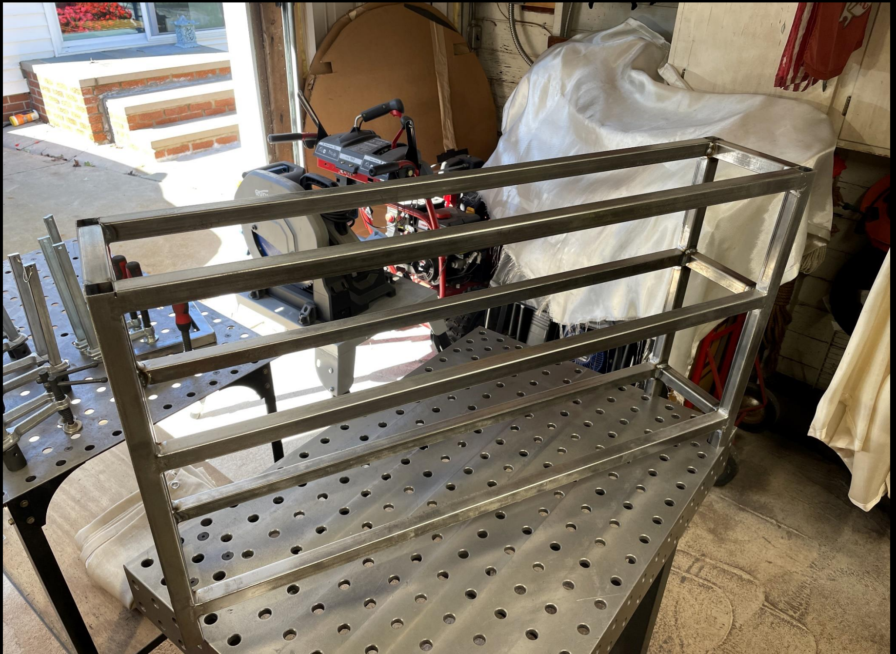
Fabrication Sequence: 15 Studio Bookshelf steel frame is welded.
