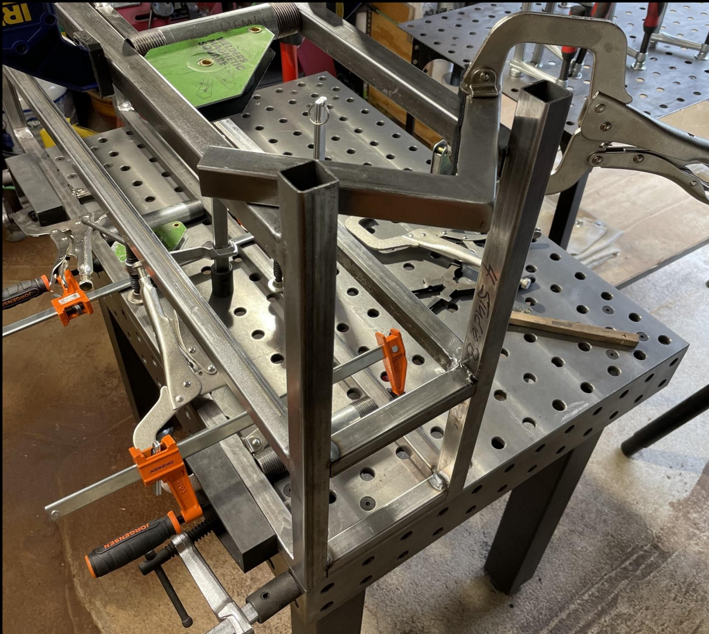
Fabrication Sequence: 13 Welding the upper cross rails locks in the panels alignment.
