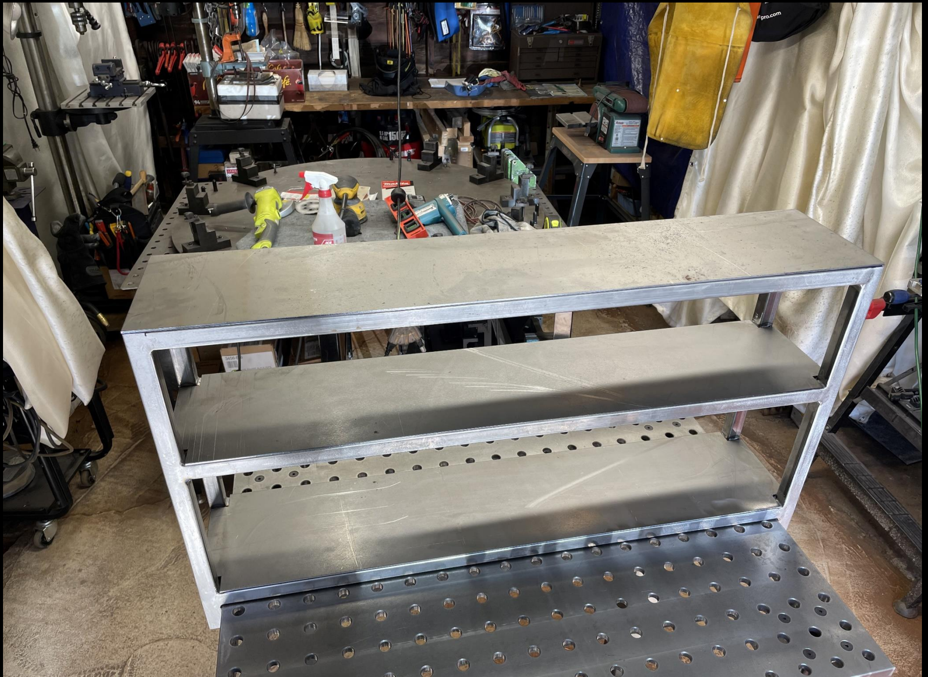
Fabrication Sequence: 17 Position & test fit the top, mid & bottom plates before welding.
