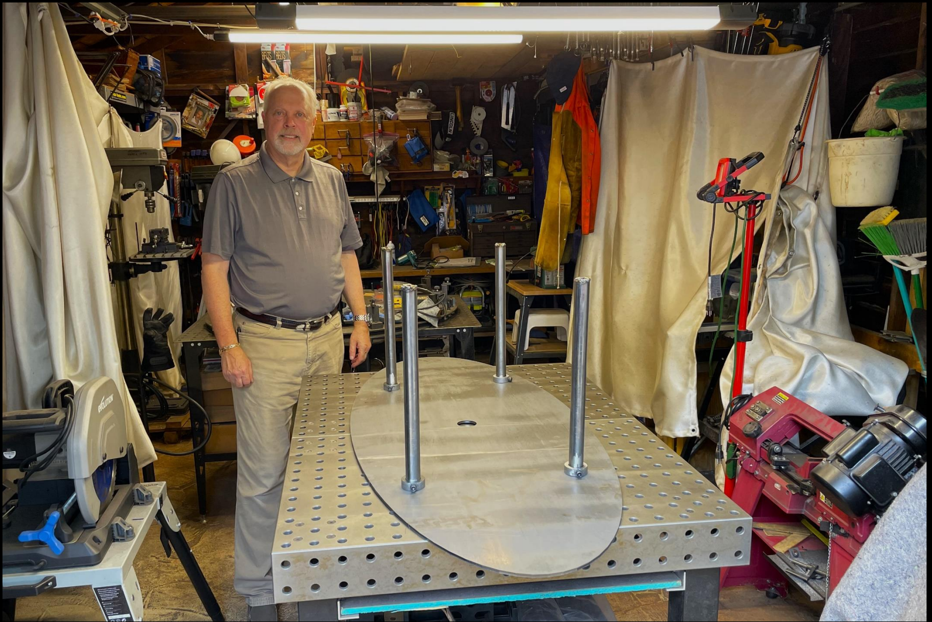
The table legs are now finished and ready to be located and welded onto the table base.
