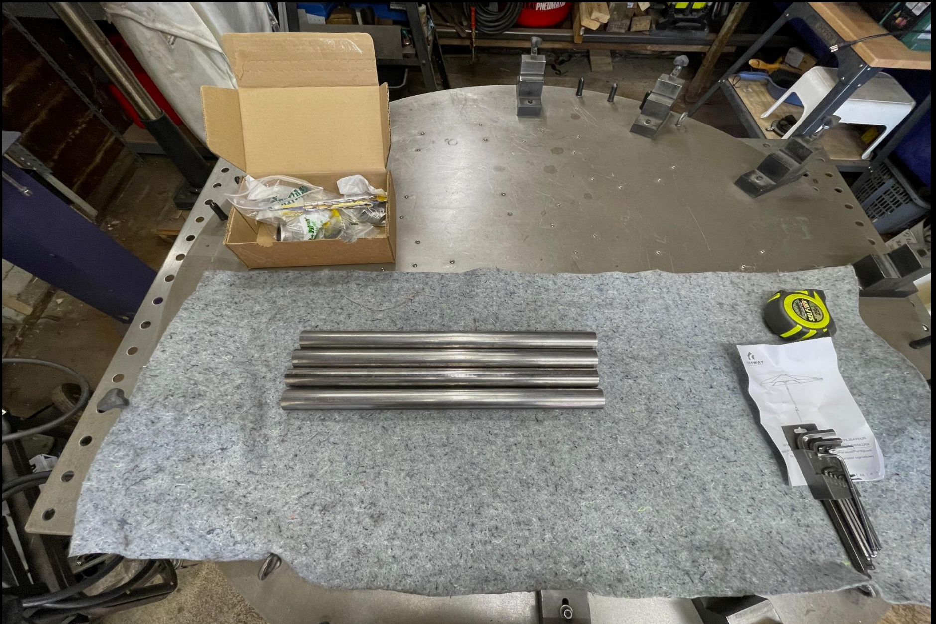
I ordered a bar of 1.25 diameter steel tube with a .120 wall thickness. I cut the bar down into 17" lengths to use for the table legs.
