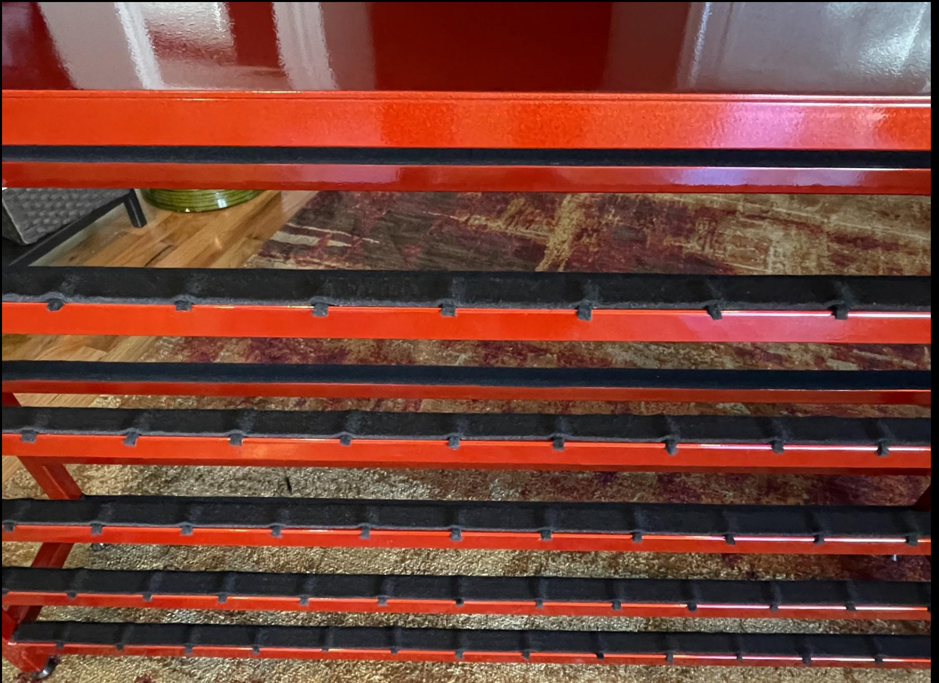
Sedona Wine Rack #12 Fabrication Sequence: 28 Felt overlay applied to cross strips
