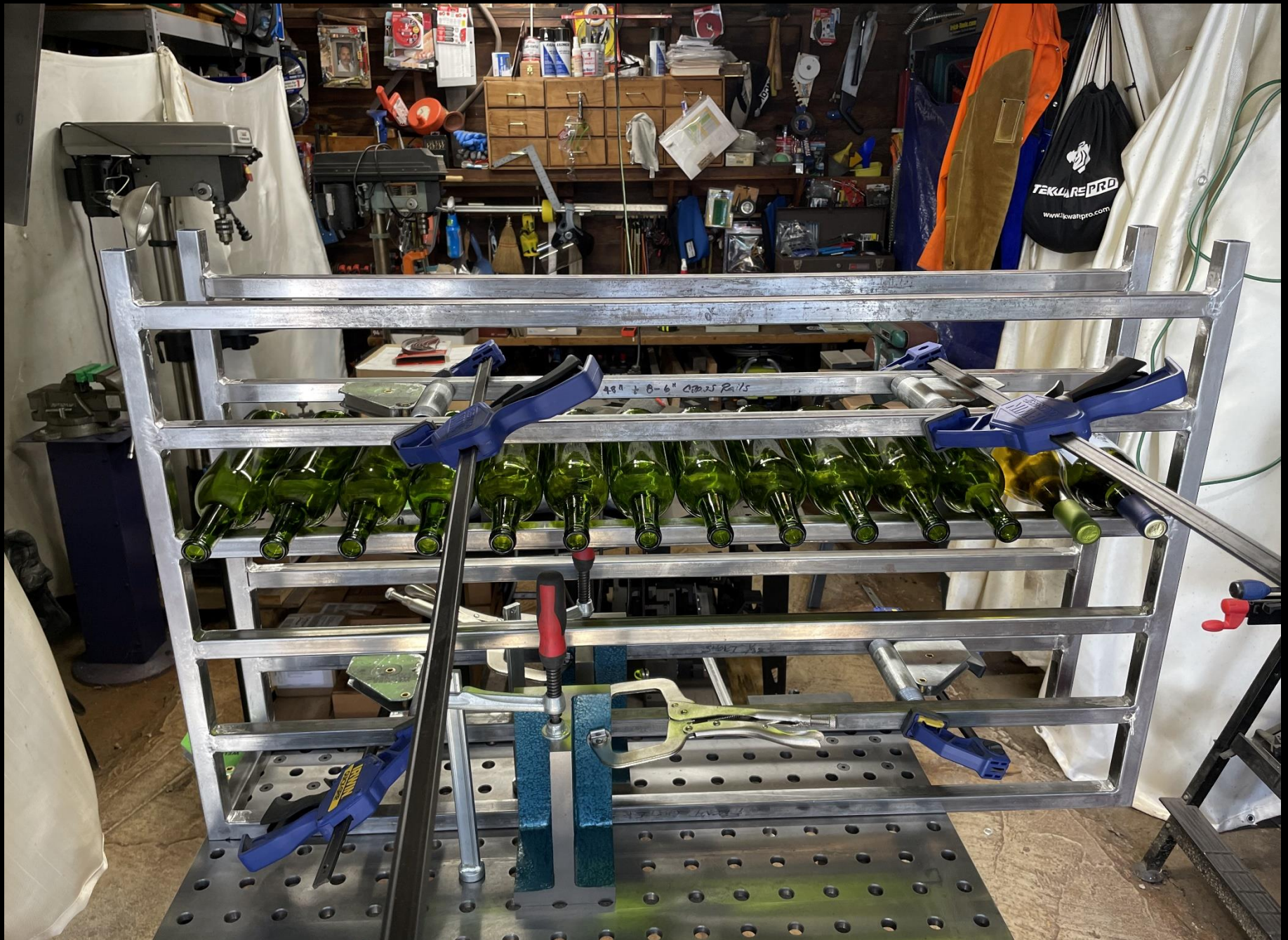
Sedona Wine Rack #12 Fabrication Sequence: 12 Bottles are loaded to check the fit
