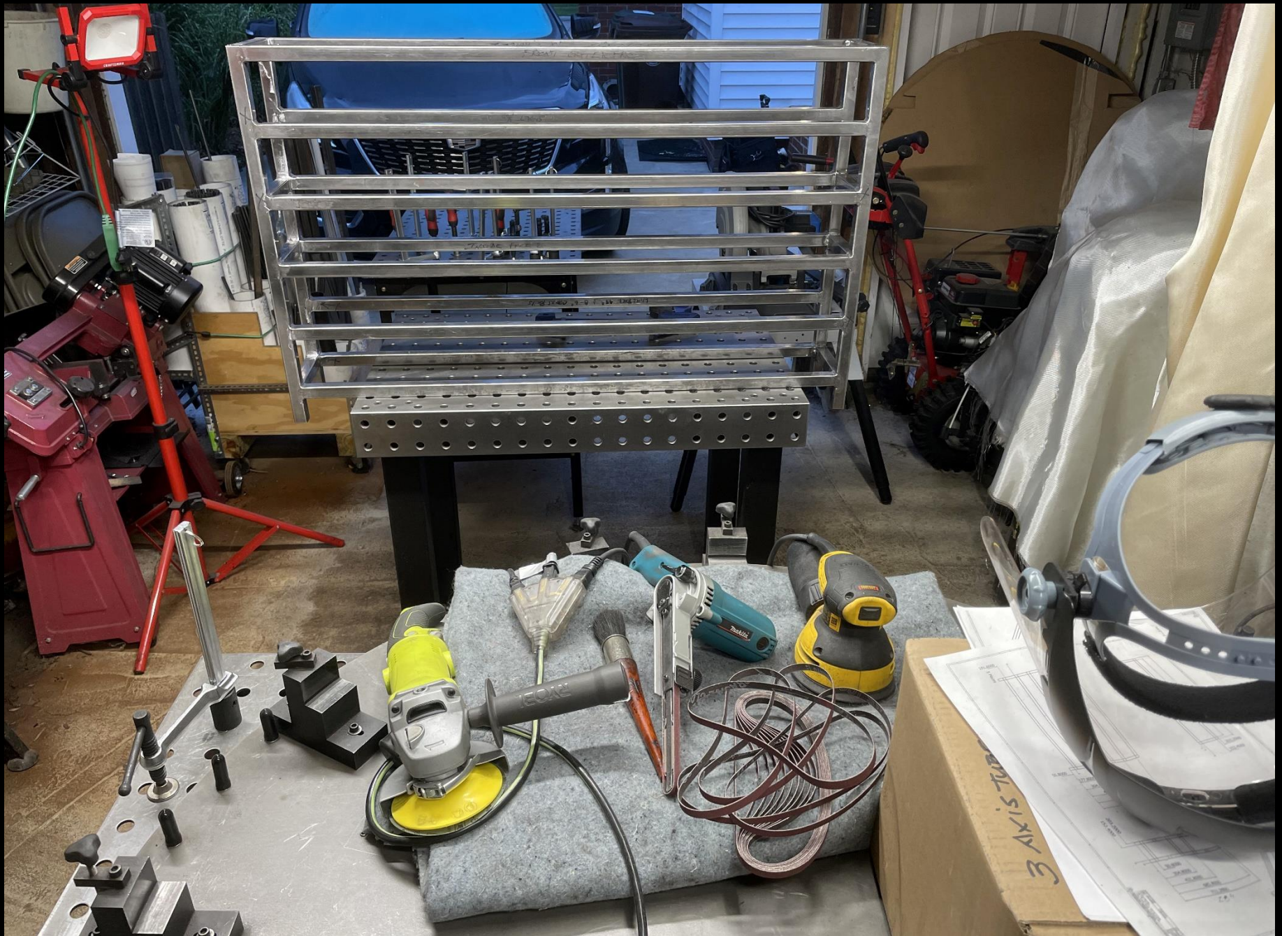
Sedona Wine Rack #12 Fabrication Sequence: 17 Clean up all cross rail welds
