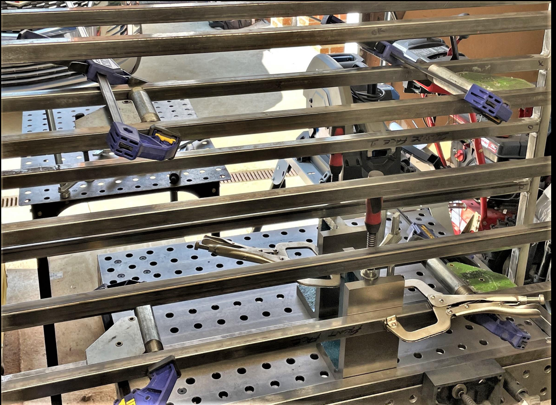
Sedona Wine Rack #12 Fabrication Sequence: 11 6" Pipe nipples keep spacing accurate
