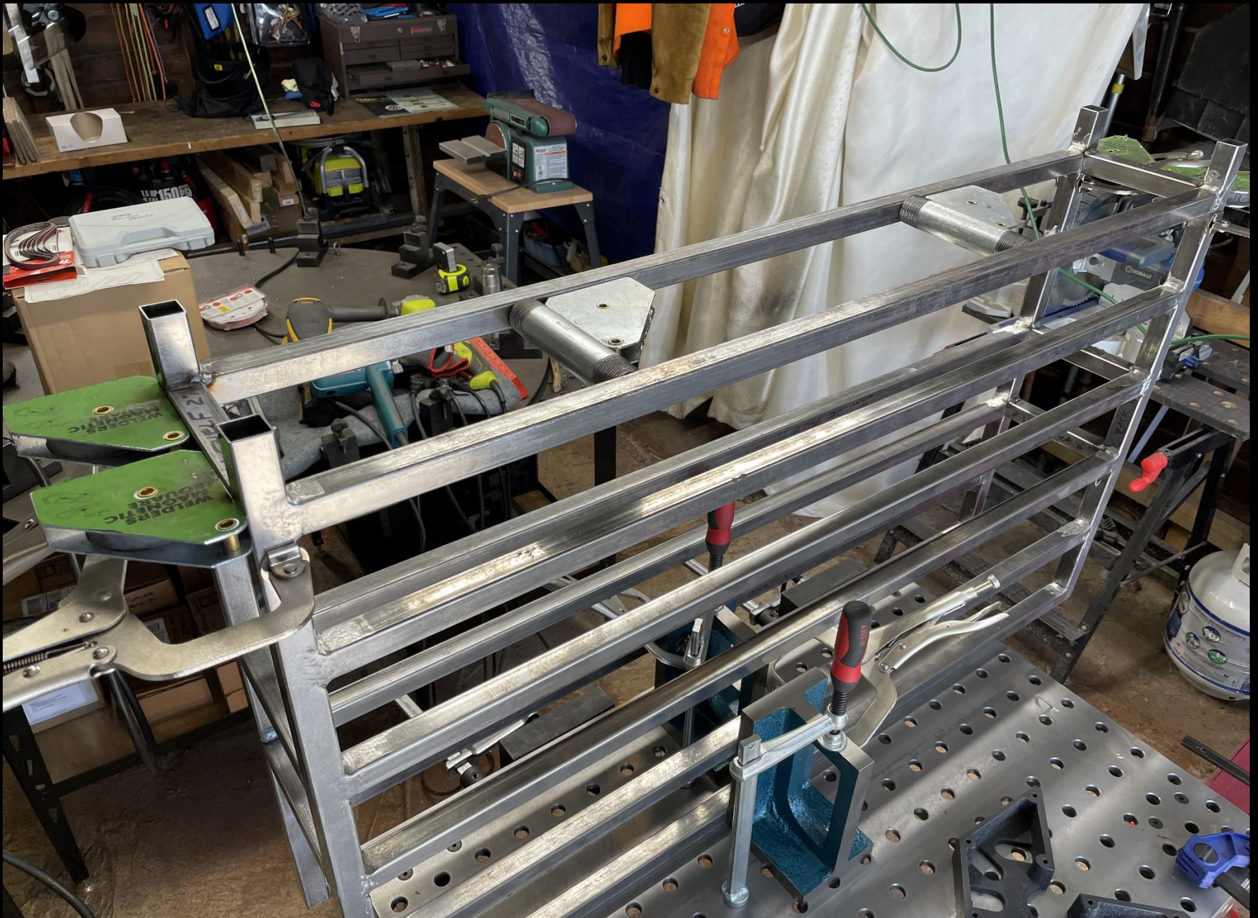
Sedona Wine Rack #12 Fabrication Sequence: 15 Bottom cross rails are welded next
