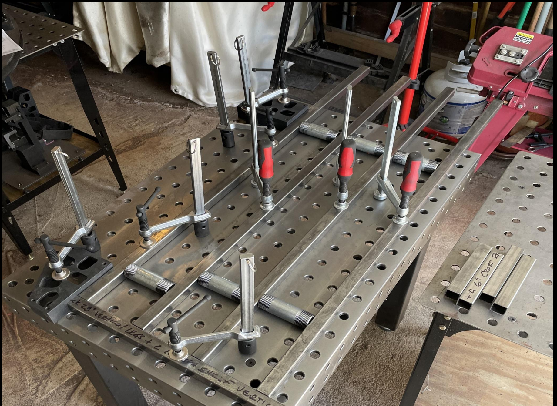
Sedona Wine Rack #12 Fabrication Sequence: 2 4" pipe nipples keep spacing accurate
