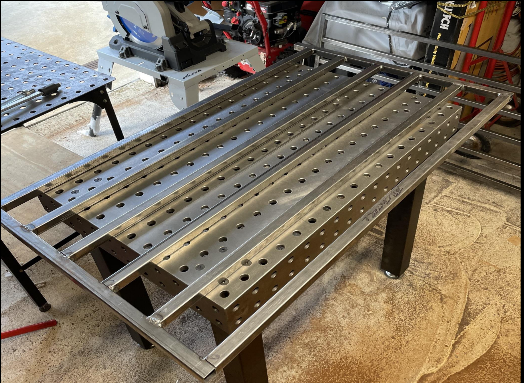
Sedona Wine Rack #12 Fabrication Sequence: 8 Panels 1 & 2 are now welded
