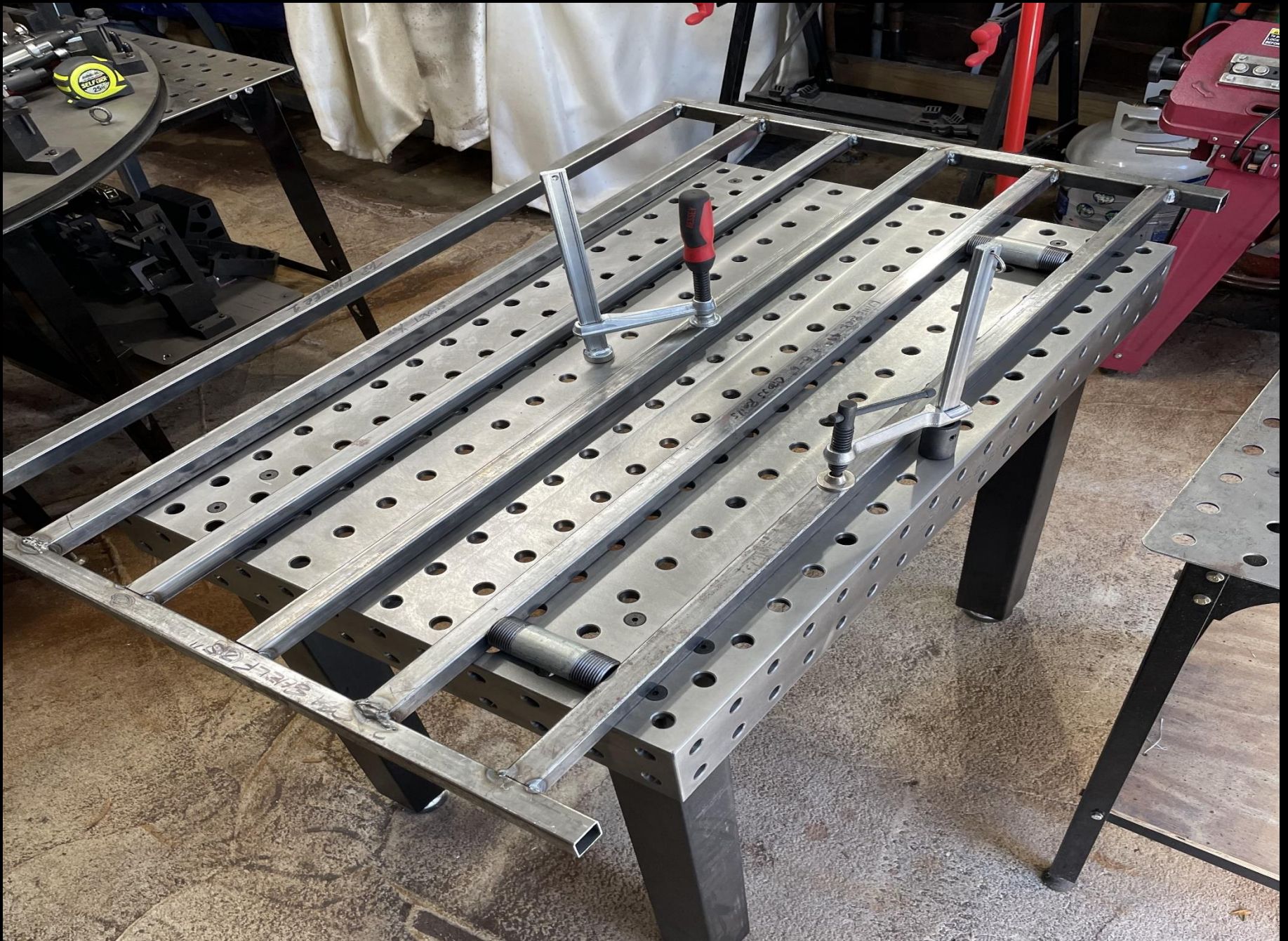
Sedona Wine Rack #12 Fabrication Sequence: 5 Bottom rail welded onto panel 1
