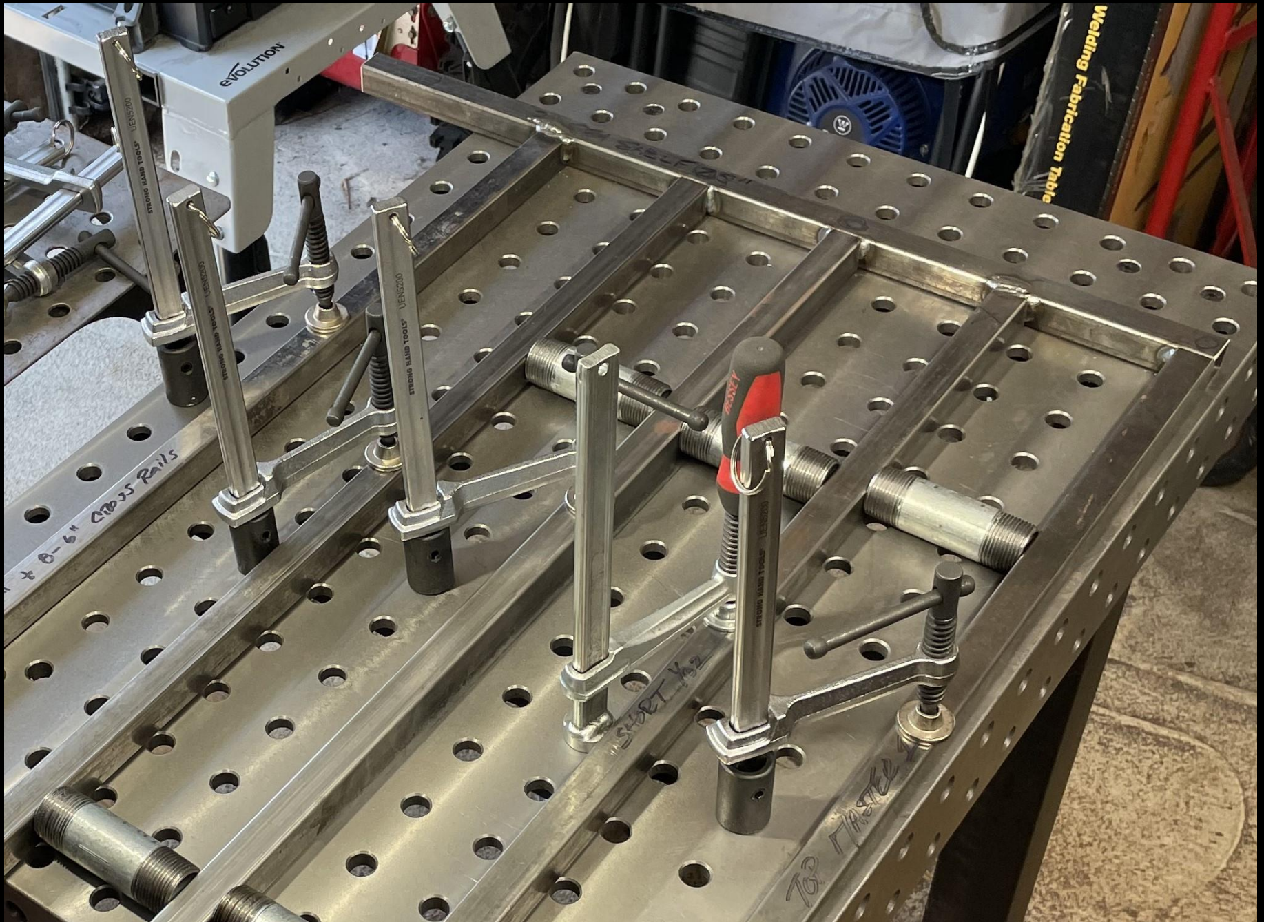
Sedona Wine Rack #12 Fabrication Sequence: 4 Inside rail welds, side 1, complete
