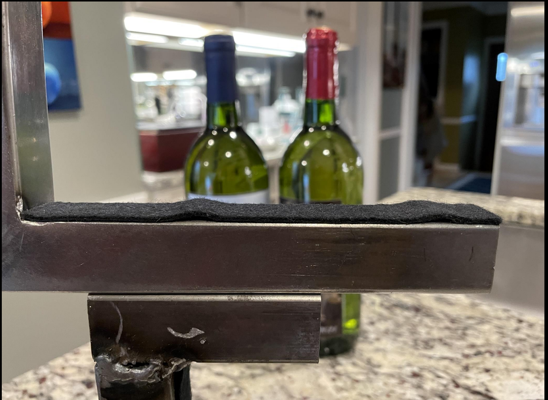
Sedona Wine Rack #12: Design mockup of felt on back rail
