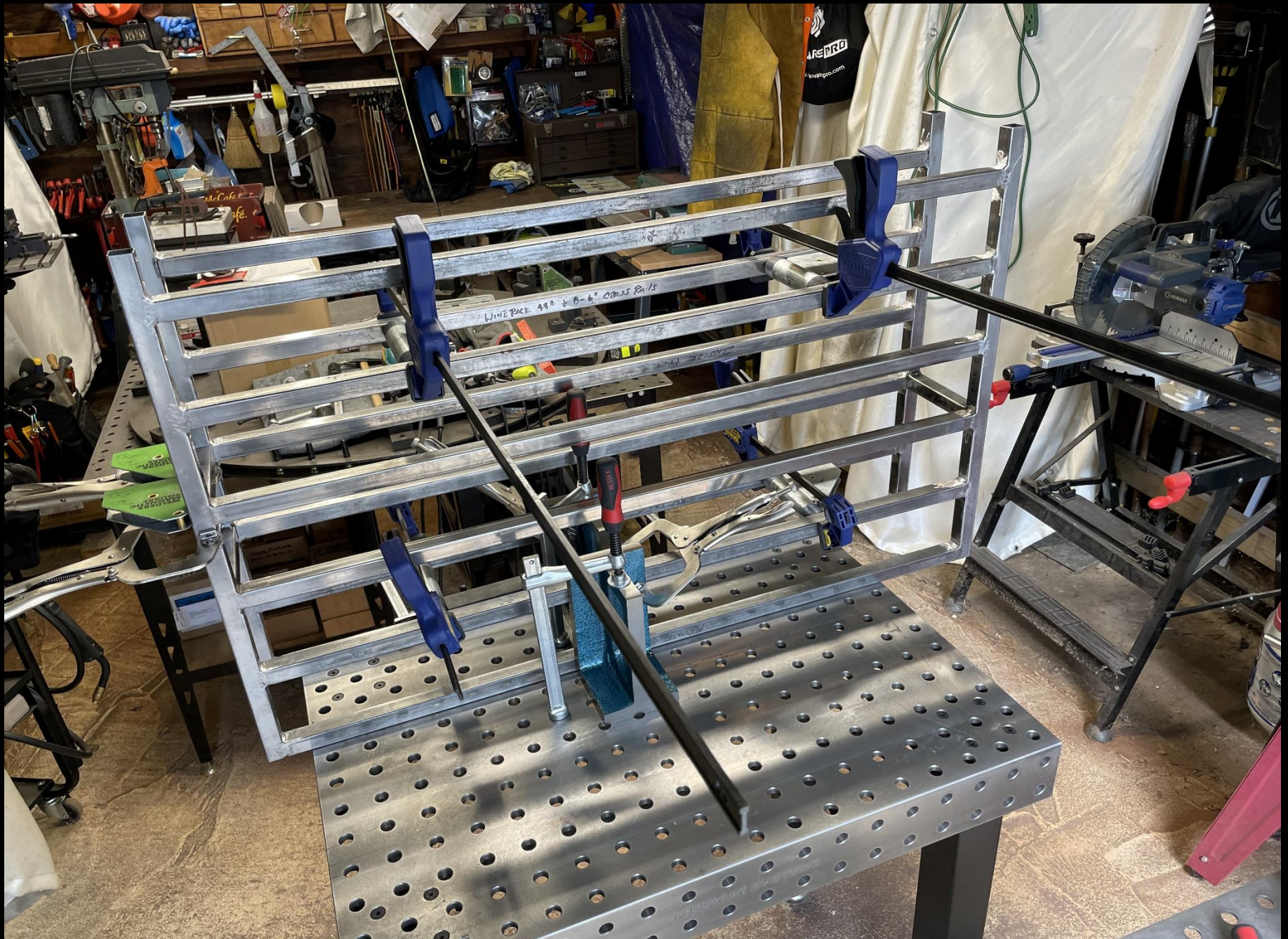
Sedona Wine Rack #12 Fabrication Sequence: 14 Mid level cross rails are welded first
