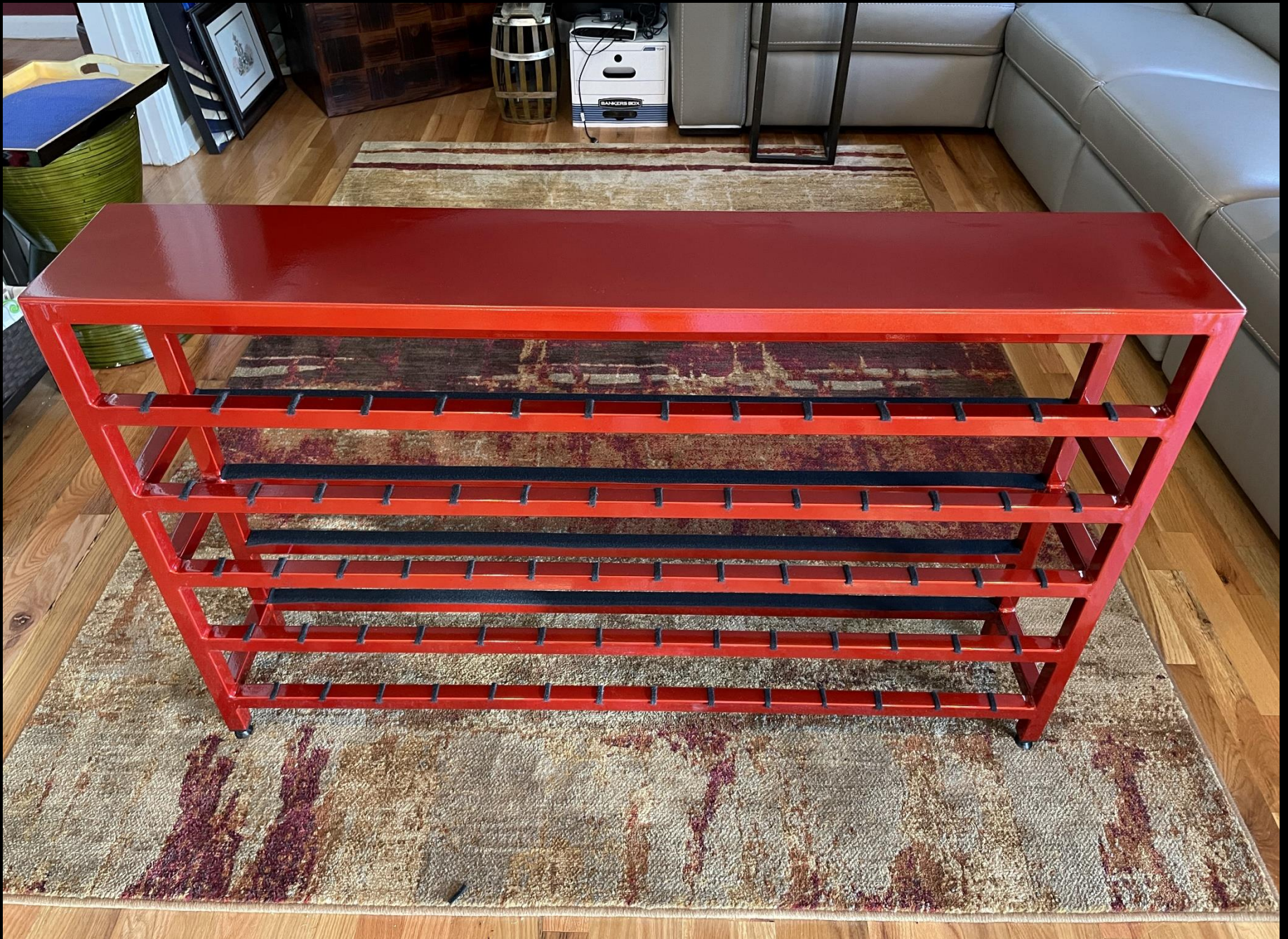
Sedona Wine Rack #12 Fabrication Sequence: 27 Felt cross strips applied to back rails
