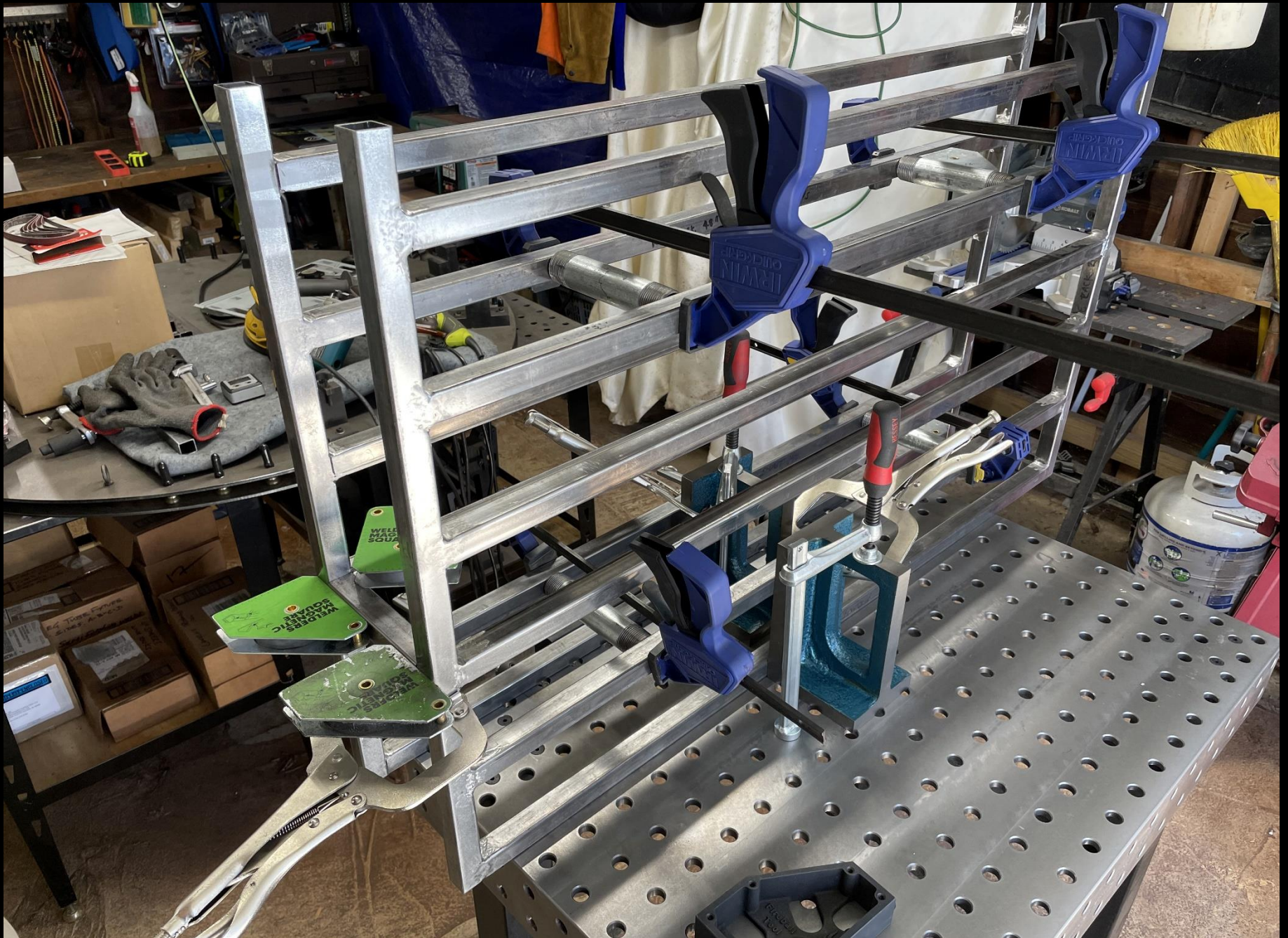
Sedona Wine Rack #12 Fabrication Sequence: 13 Locating cross rails for welding
