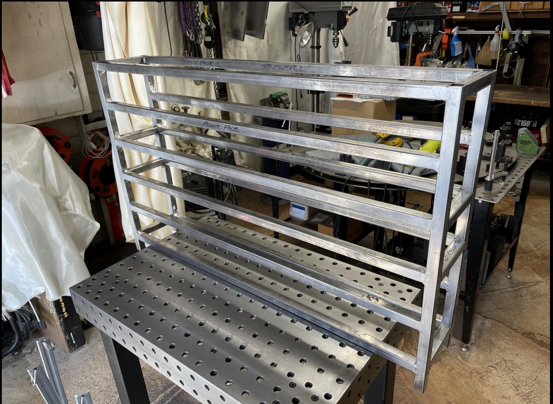
Sedona Wine Rack #12 Fabrication Sequence: 16 Top cross rails are welded last
