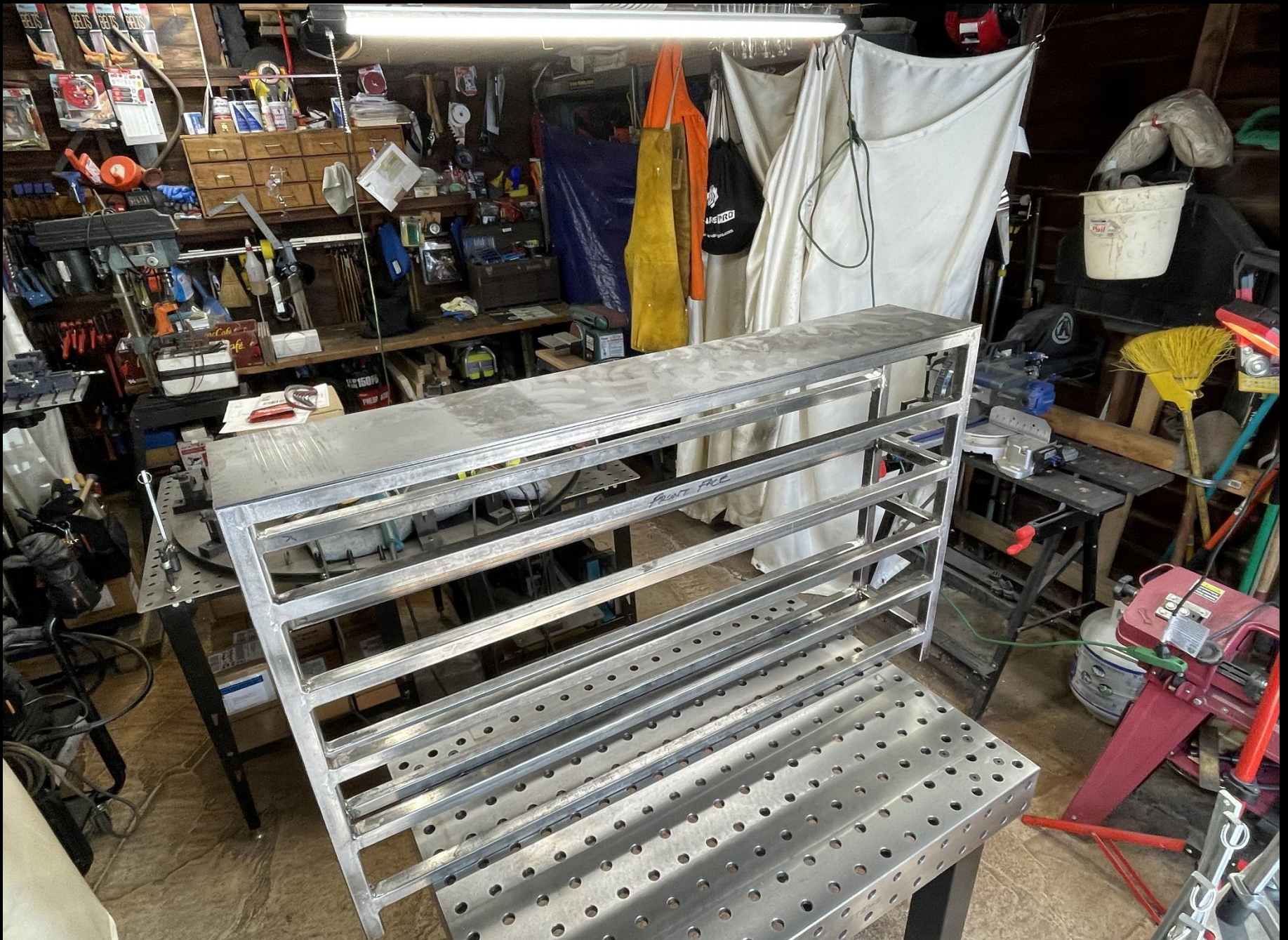
Sedona Wine Rack #12 Fabrication Sequence: 18 Check top shelf for fit & flatness
